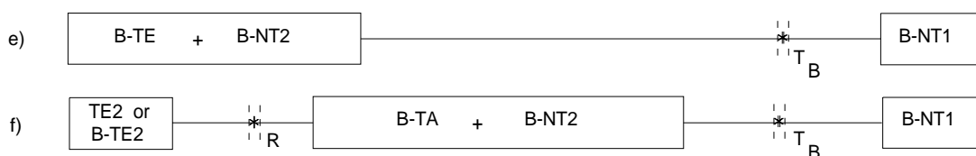
Configurations where B-ISDN physical interfaces occur at reference point T_B only
