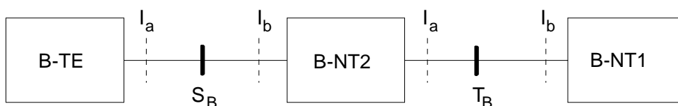
Figure 4: Reference configuration at reference points S_B and T_B
