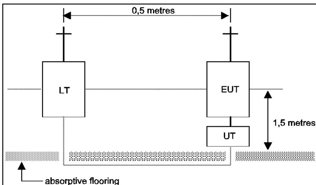
Figure 14: Test arrangement
