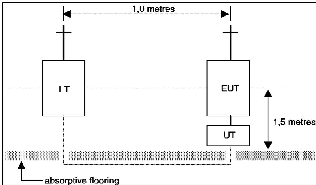
Figure 15: Test arrangement
