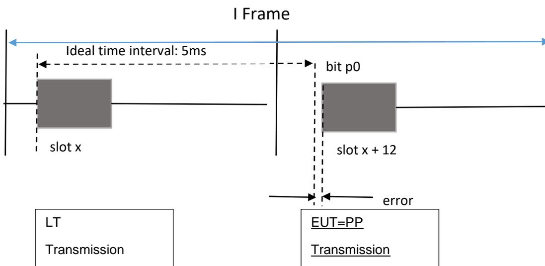
Figure 24: PP packet transmission error definition
