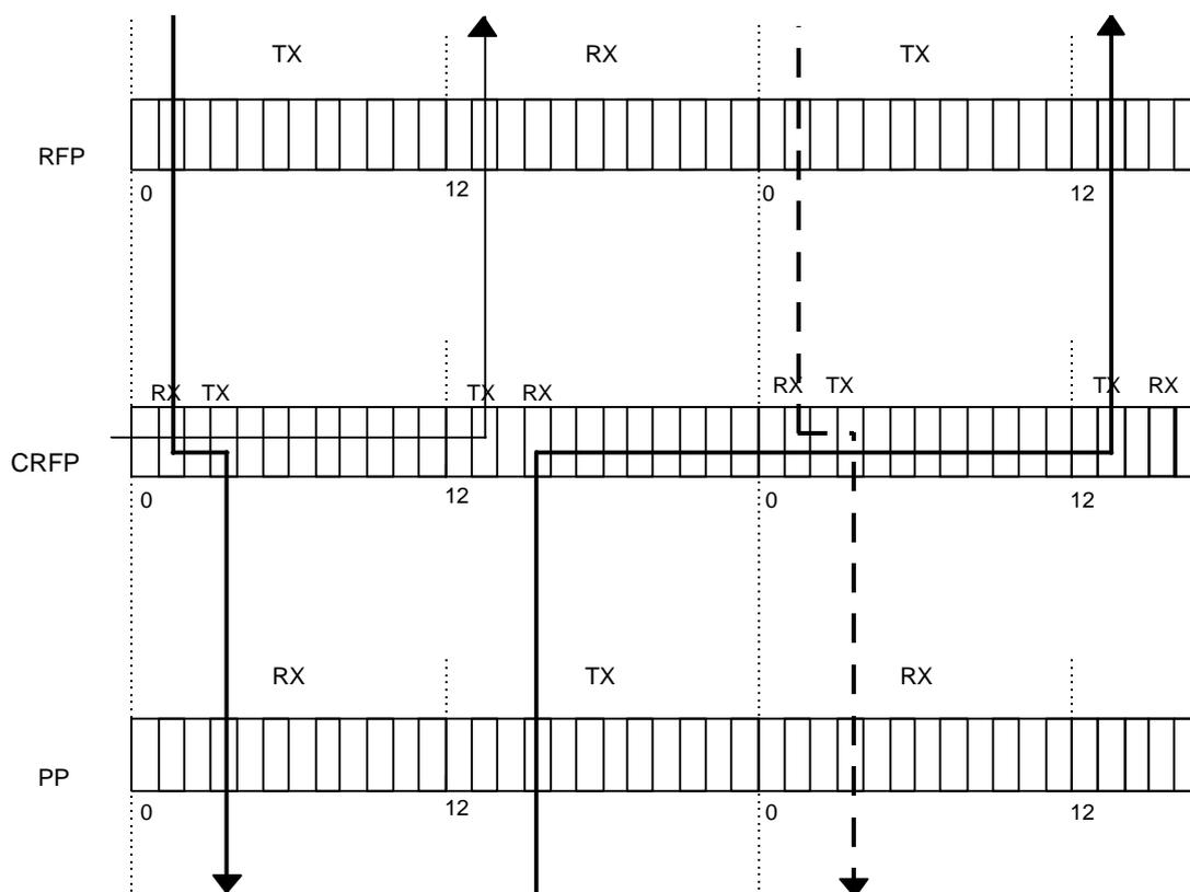
Figure 37: Typical frame multiplexing structure of the CRFP
