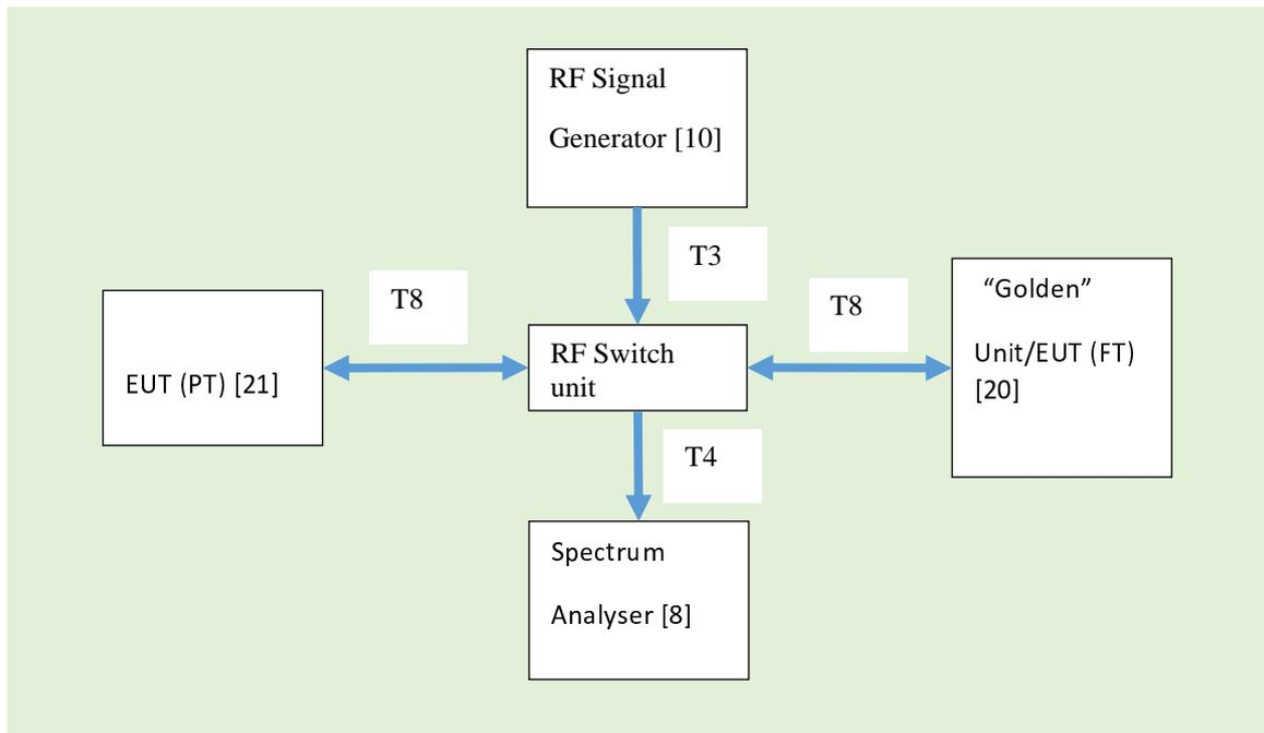
**Figure 33: PT Test Setup**
