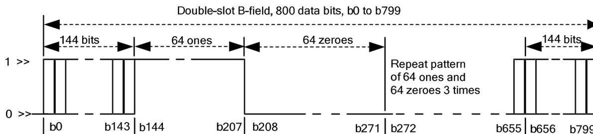
NOTE: Bits  $b_0$  to  $b_{143}$  and  $b_{656}$  to  $b_{799}$  are alternating 1s and 0s.
