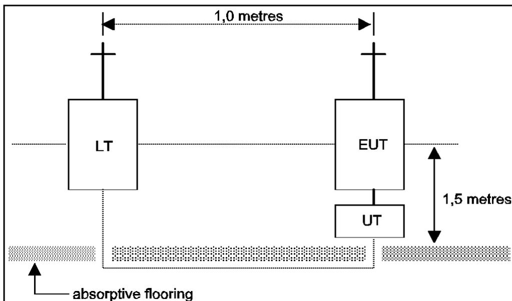
Figure 16: Test arrangement
