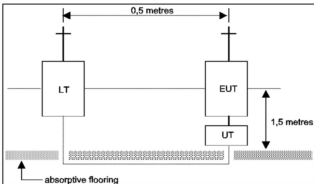
Figure 15: Test arrangement
