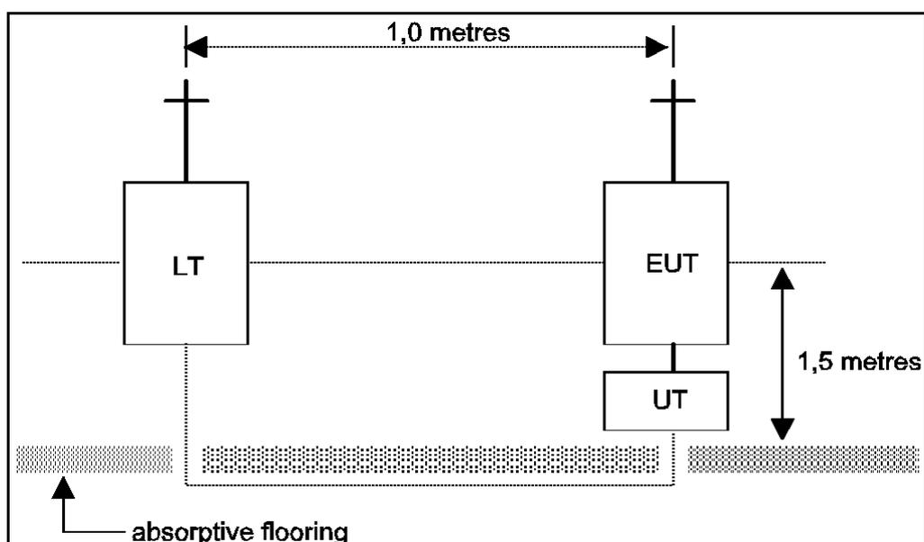
Figure 16: Test arrangement
