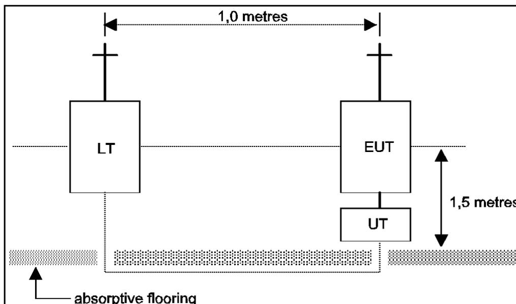
Figure 17: Test arrangement
