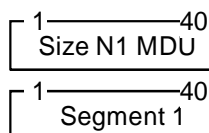
Figure 11.6.3.4.2: Segmentation of Size N1 MDU
