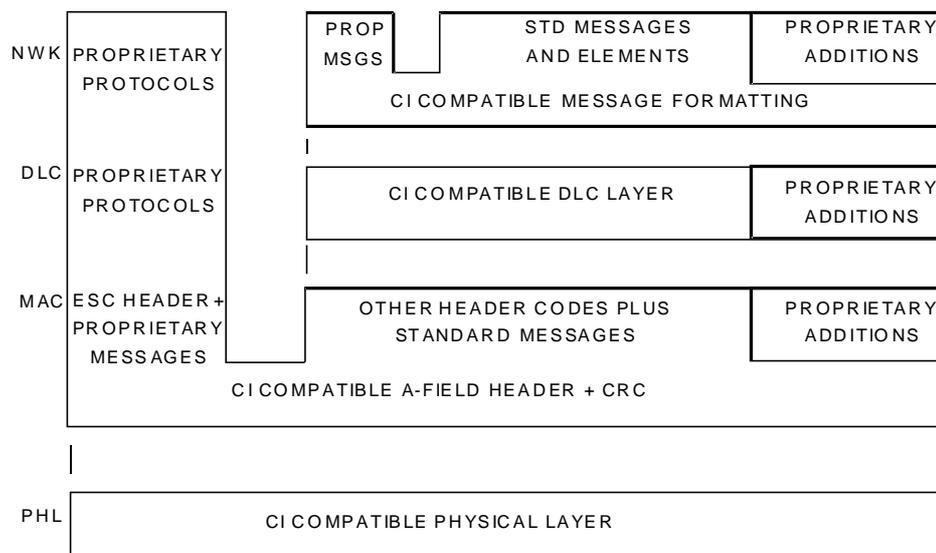
**Figure 2: Structure of escape routes within the CI**
