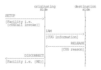
Figure A.4: Call fails destination network side checks
