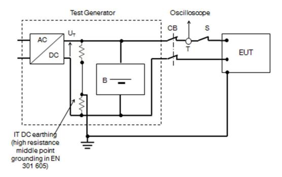
Figure 4: Inrush current test set-up
