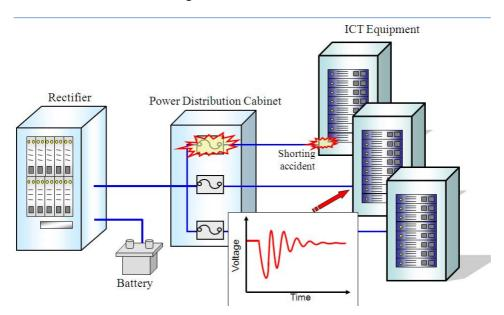
Figure F.1: Definition of transient voltage impact
