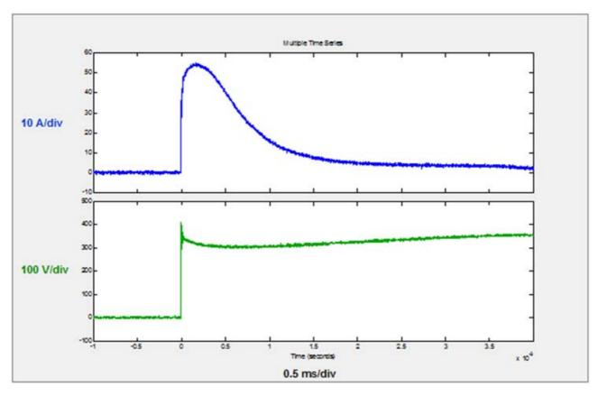
Figure D.2: Example of inrush current measured on small ICT equipment
