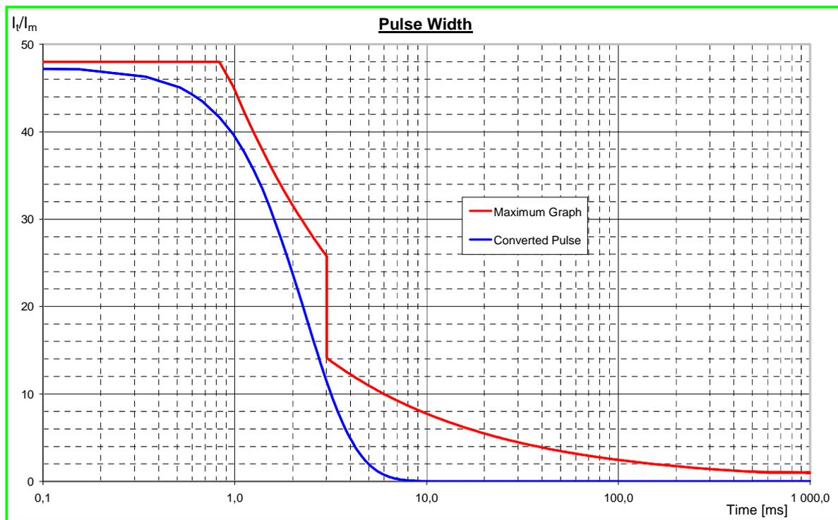
**Figure C.2: Example of values for a typical inrush current ratio plotted against limit curve**
