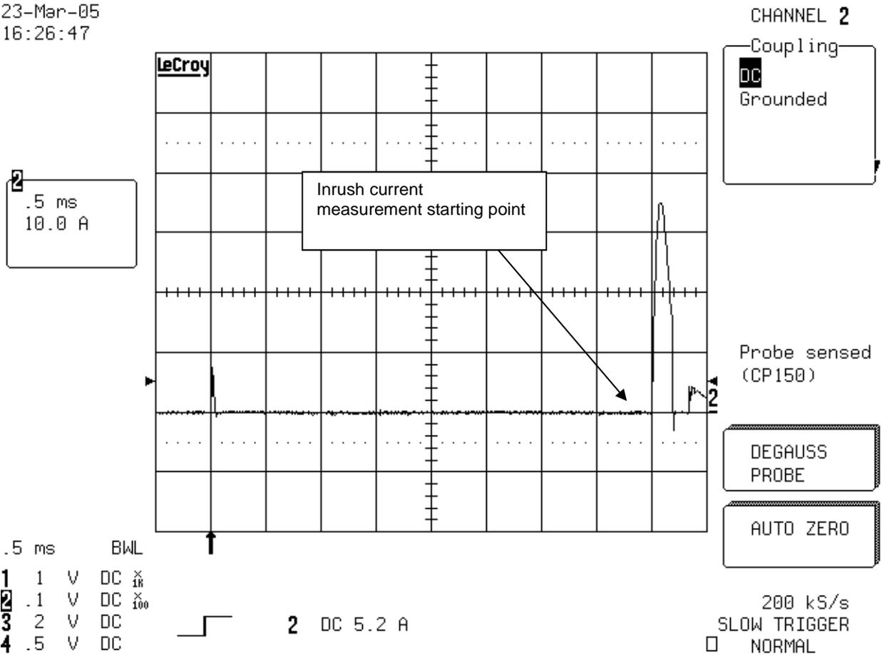
NOTE: In this example the inrush current measurement starting point is set at the beginning of the biggest pulse.
