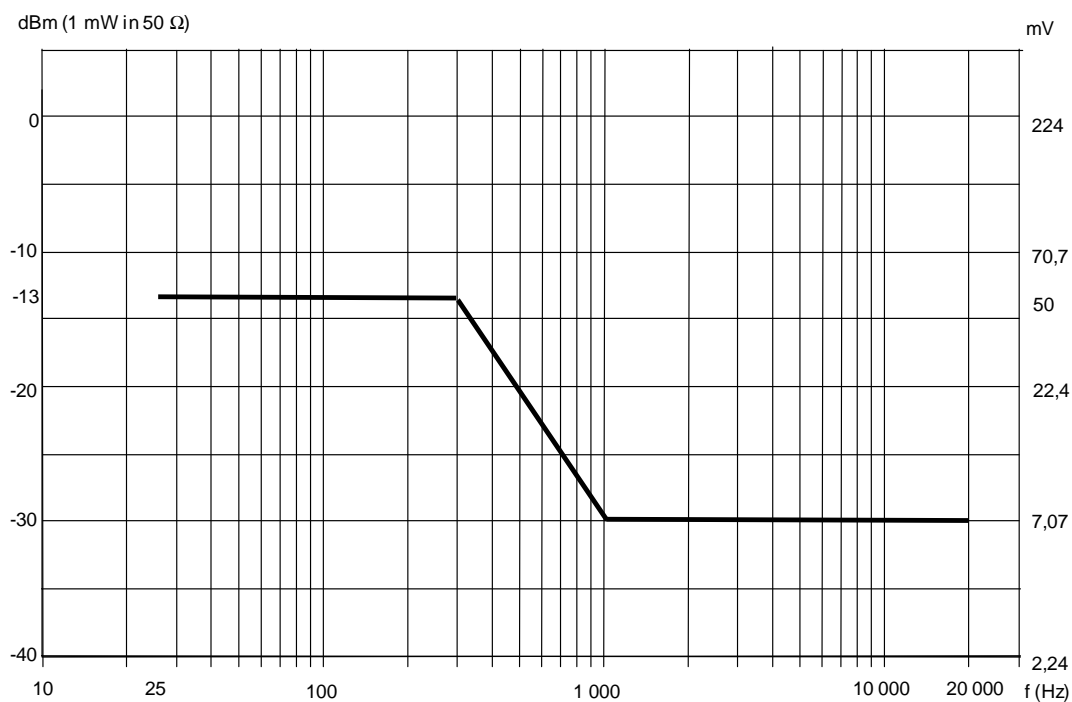
Figure 5: Immunity level of narrow-band noise at interface "A"
