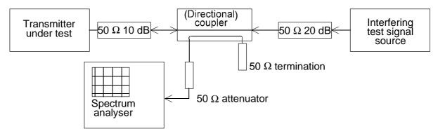
Figure 11: Measurement arrangement
