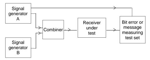
Figure 25: Measurement arrangement
