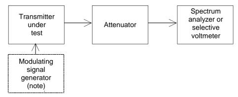
NOTE: Used only if it is not possible to perform the measurement with the transmitter unmodulated.
