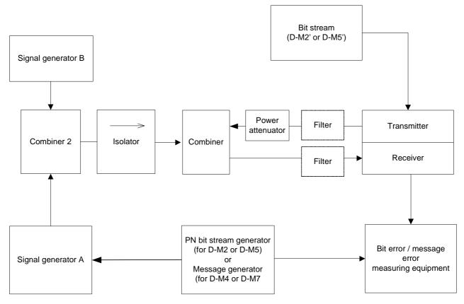
Figure 36: Measurement arrangement for equipment without a Duplex filter
