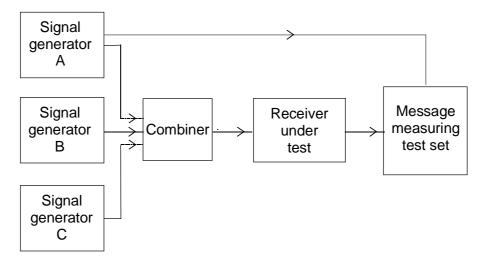
Figure 27: Measurement arrangement
