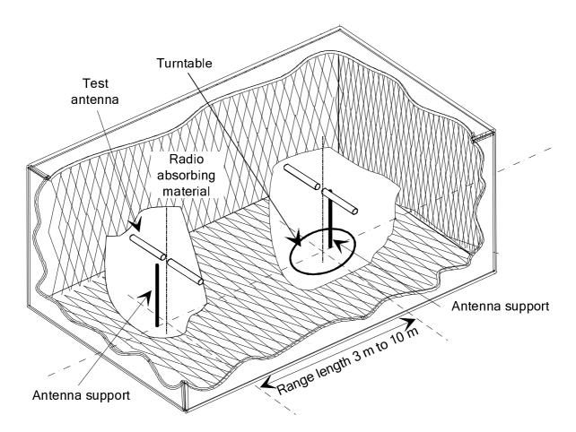
Figure A.1: A typical anechoic chamber
