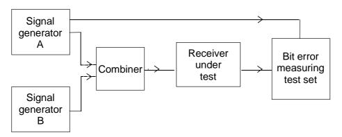
Figure 28: Measurement arrangement
