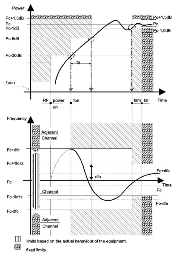
Figure 12: Transmitter attack time according to clause 7.7.1 a) and transient behaviour during switch-on (case where the attack time is given by the behaviour of the power rise)
