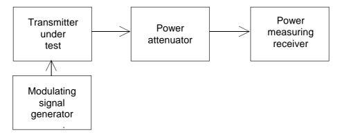
Figure 7: Measurement arrangement
