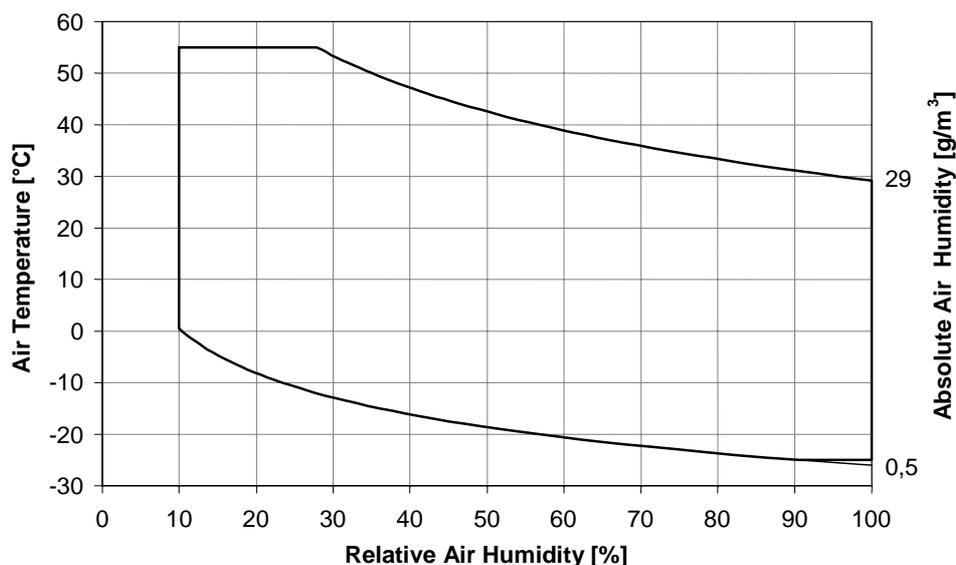
Figure 3: Climatogram for class 3.3: Not temperature controlled locations
