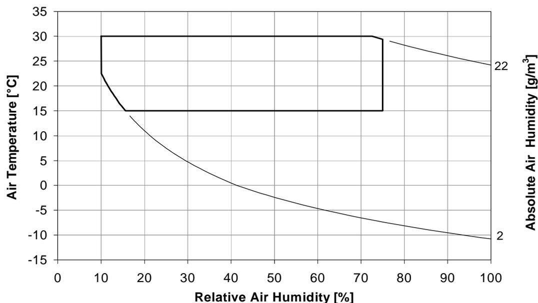
Figure 6: Climatogram for Class 3.6: Telecommunication control rooms
