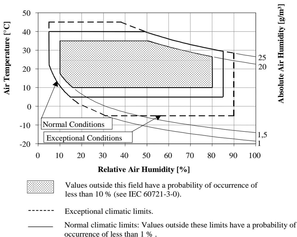
NOTE: Exceptional conditions may occur following the failure of the temperature controlling system. This is described as 3.1E in the tables but it should be noted that there is no separate class 3.1E.
