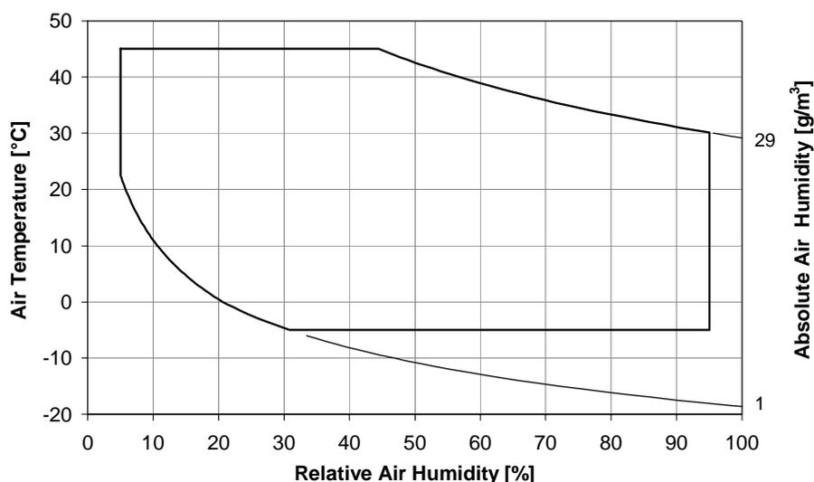
**Figure 2: Climatogram for class 3.2: Partly temperature-controlled locations**
