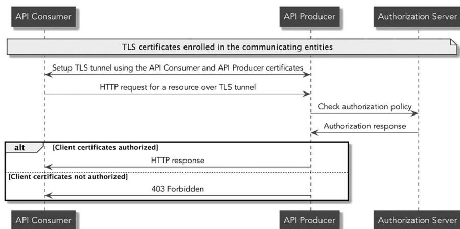
**Figure 4.4.4.3-1: Flow of API authorization using TLS certificates**
