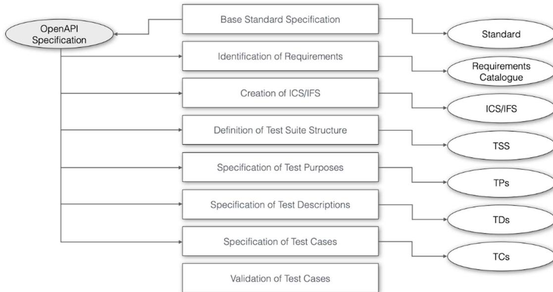
**Figure 5.4.2-1: RESTful API Test Specification Process with OpenAPI**
