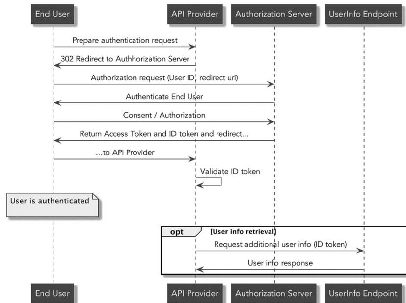
Figure 4.4.4.4-1: Flow of API authorization using OpenID connect
