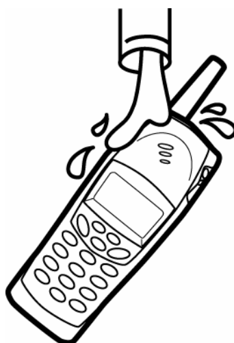
Figure 3: Bad example of an illustration (can be misunderstood as the mobile terminal should be washed). This illustration would need an explanatory text or an over-crossing.
