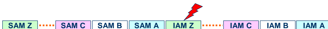
Figure 18: Sample MSU sequence from figure above on single M2PA link forming one link set
