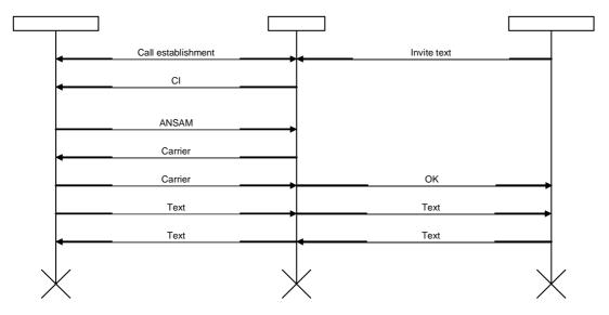
Figure 9: Example 2 - Call from IP to carrier based textphone, text only or preferred
