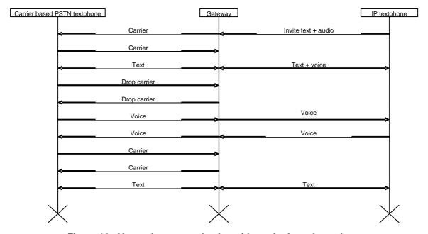
Figure 12: Alternating text and voice with carrier based textphone
