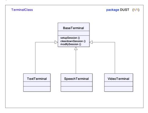
Figure 1: UML diagram showing text, speech and video terminals as specializations of a base terminal
