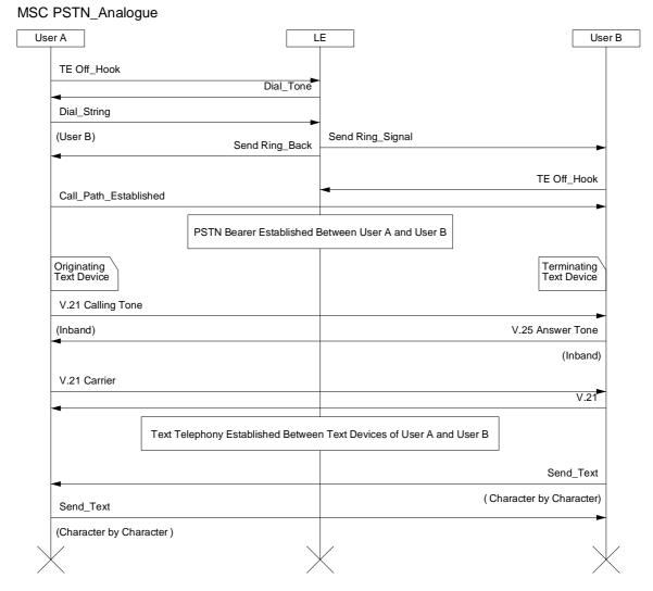
Figure A.2: PSTN Carrier Text Telephone Call Establishment
