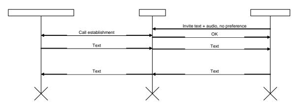
Figure 11: Example 5 - Call from IP without text preference to carrier less textphone
