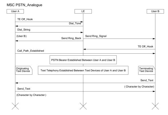
Figure A.3: PSTN Carrier-less Text Telephone Call Establishment
