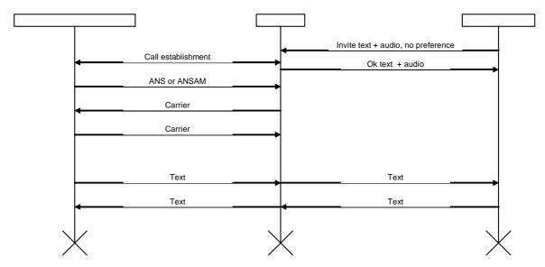
Figure 10: Example 4 - Call from IP to carrier based textphone, no text preference
