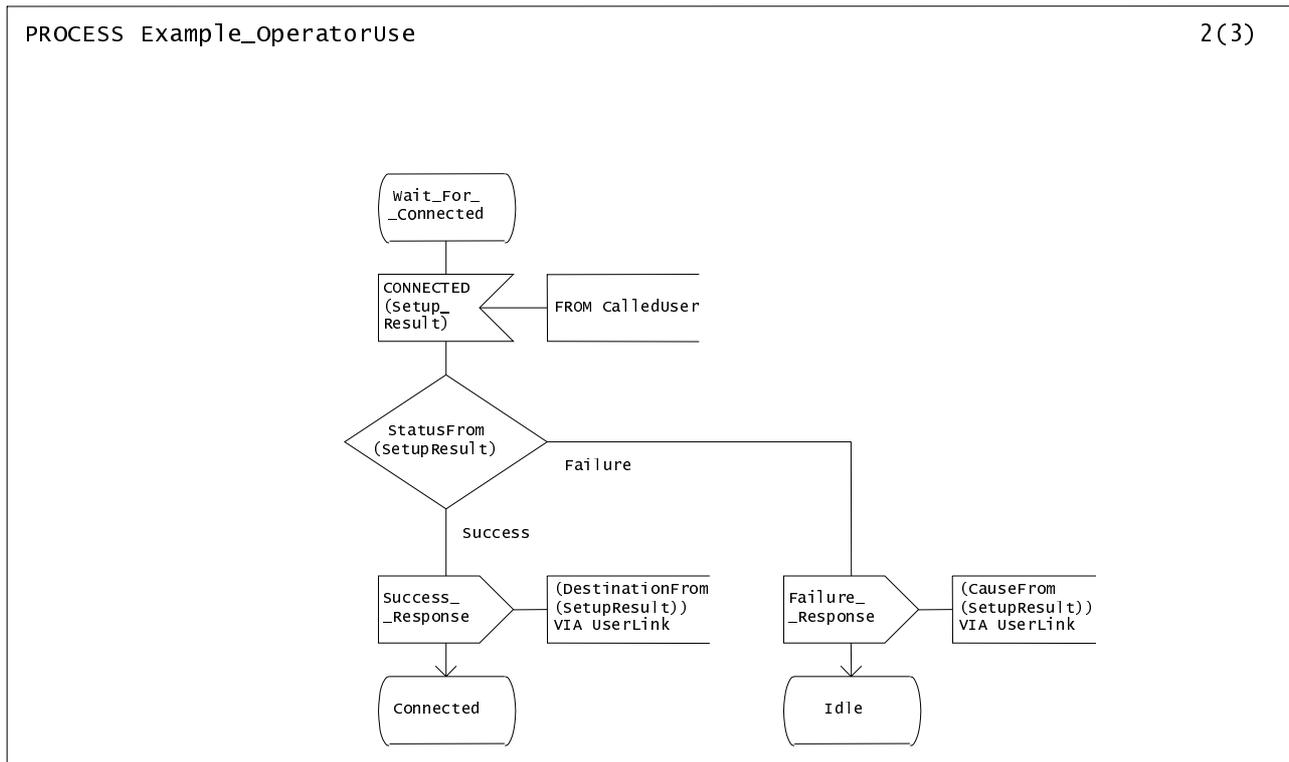
**Figure 32: Examples of operator invocation**
