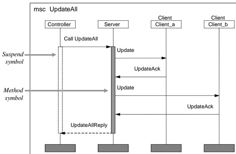
**Figure 91: Specification of synchronous communication utilizing the suspend symbol and the method symbol.**
