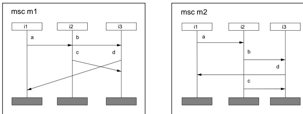
Figure 85: Clear ordering of events and separation of message lines
