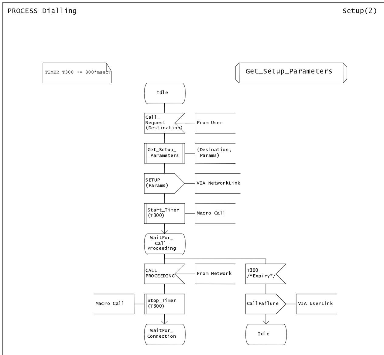
Figure 36: Process illustrating the use of macros
