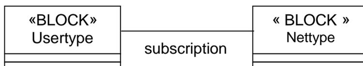
**Figure 60: A named association between two block types**
