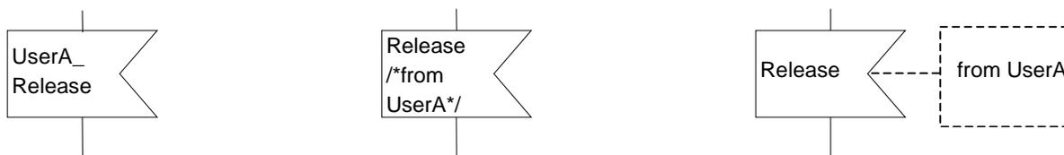
**Figure 68: Identifying the source of an input signal**
