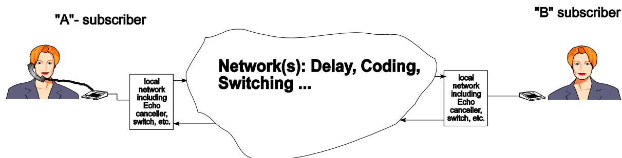
Figure 2: Typical test setup for determining the speech transmission quality from end-to-end (mouth-to-ear) by subjective evaluation of the speech quality relevant parameters (example for handset/hands-free communication)
