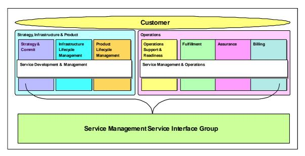
Figure 10: Service Management Service Interface Group compared with eTOM
