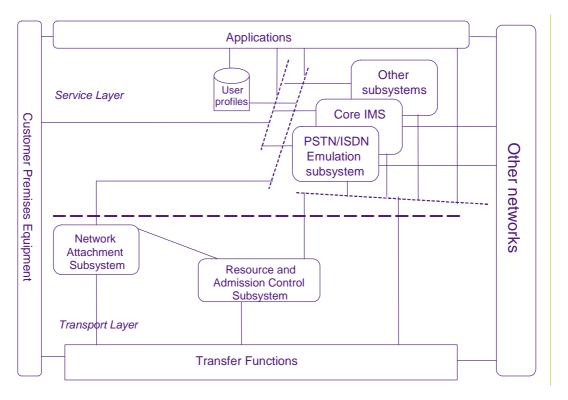
Figure 2: NGN Architecture components
