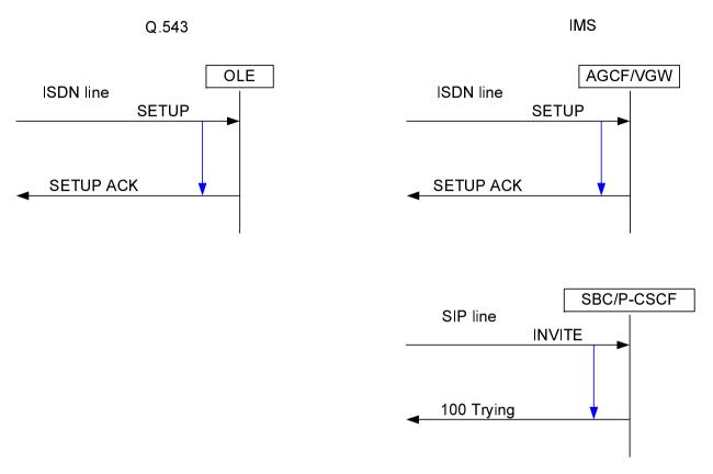
Figure 2: Local exchange ISDN subcribercall request delay: overlap sending
