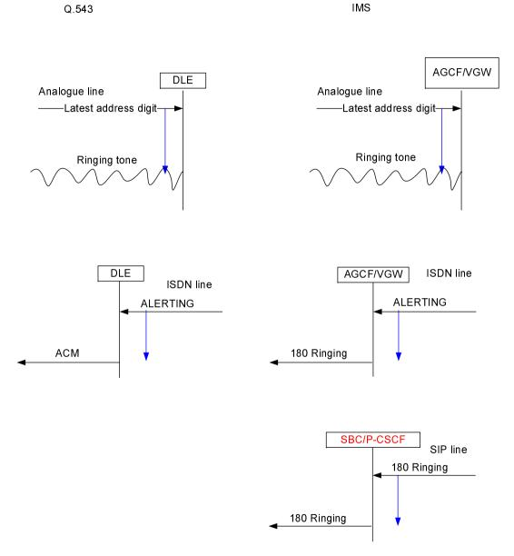
Figure 4: Local exchange Alerting sending delay for terminating traffic (in different locations)
