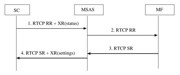
Figure A.16: RTCP signalling for the exchange of synchronization status and settings instructions for a CoD service
