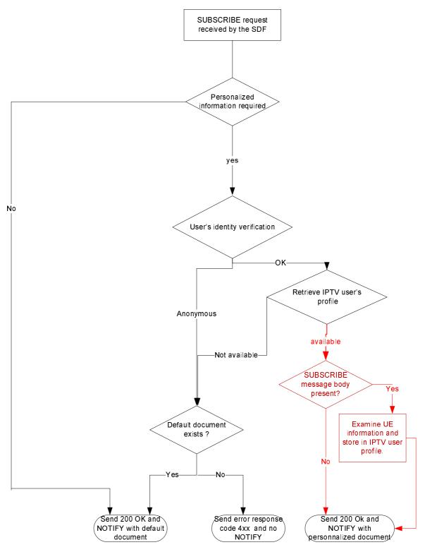
Figure 5.2.2.2: SDF logic for processing SUBSCRIBE requests
