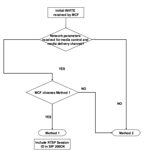
Figure Q.2: MCF-side RTSP method decision logic
