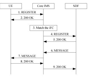
Figure A.2: Service discovery of Push mode operation
