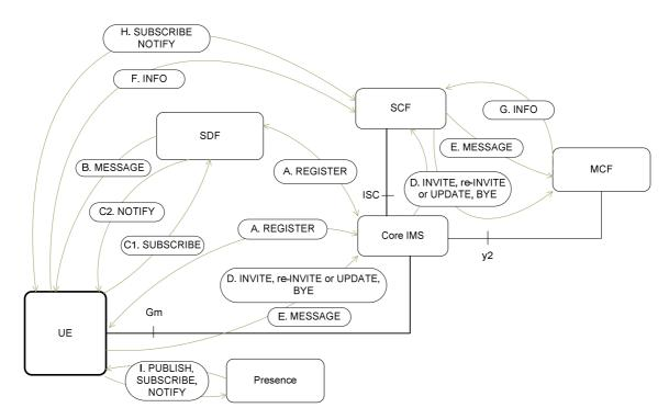
Figure H.1: IMS based IPTV - SIP protocol model
