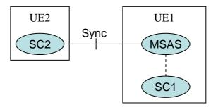
Figure A.17: UE acting as MSAS for inter-destination media synchronization between UEs
