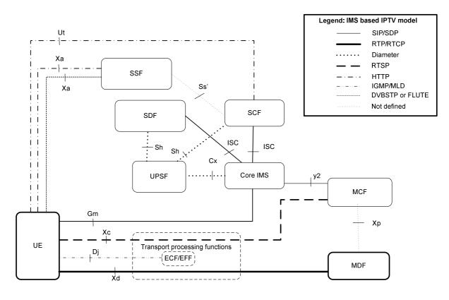
Figure 4.1: Protocols used in functional architecture for the IMS-based IPTV service
