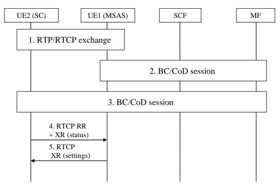
Figure A.18: RTCP signalling for the exchange of synchronization status and settings instructions between UEs directly
