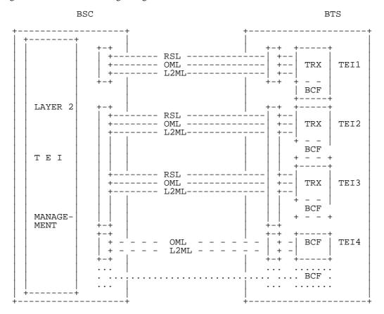
Figure 7.2: Logical L2 links of A-bis interface
