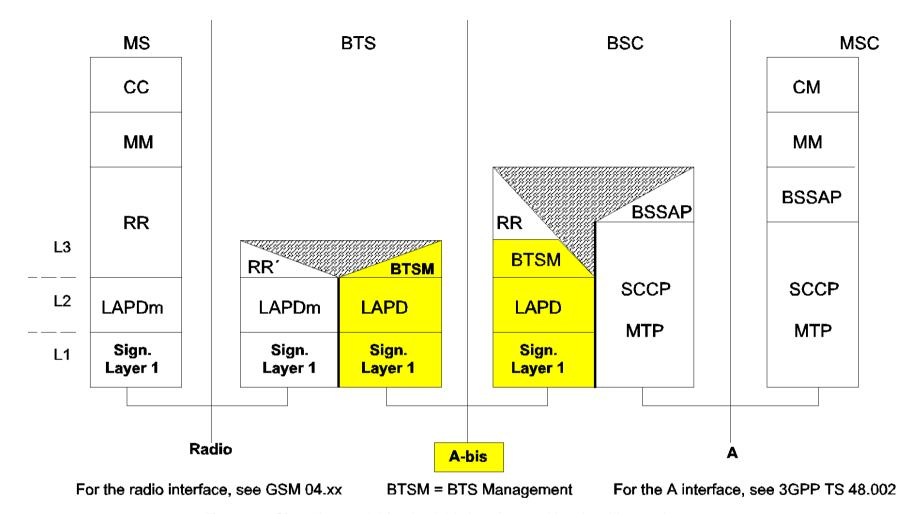
Figure 7.3: Signalling model for the A-bis interface and its signalling environment
