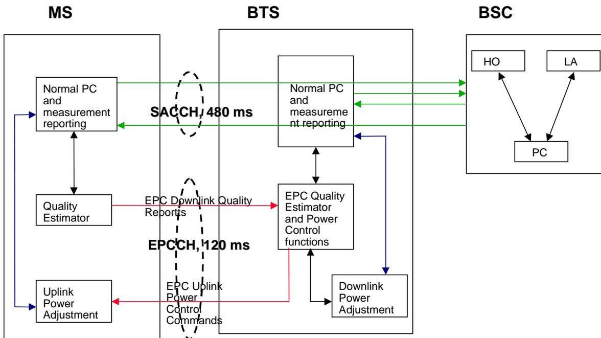
The BSC has the control over which power control loop is in use. For the uplink power control, this is signalled with one control bit on the Abis interface to the BTS, which in turn informs the MS, when the enhanced power control shall be used.
