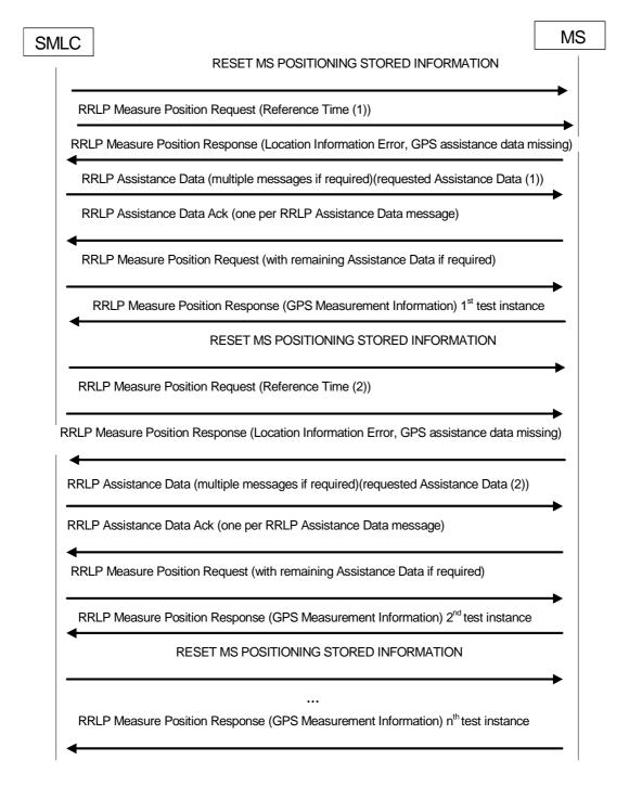
Figure M.5-2: MS-Assisted A-GPS Message Sequence
