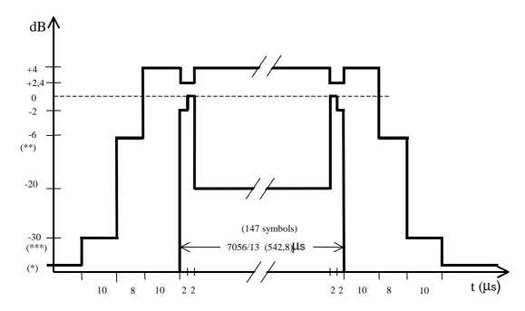
Figure B.2: Time mask for normal duration bursts (NB) at 8-PSK modulation
