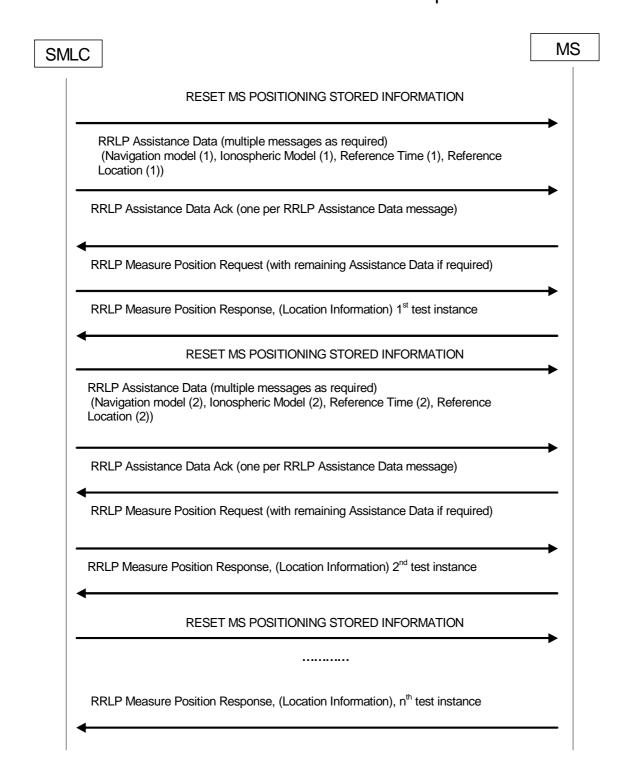
Figure M.5-1: MS-Based A-GPS Message Sequence
