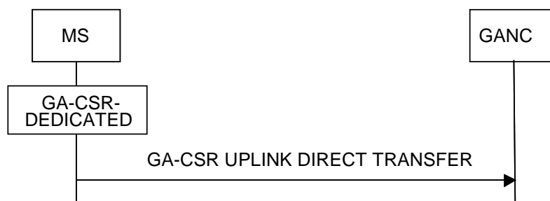
Figure 7.2.1.1 Uplink Direct Transfer, normal flow
