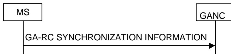
Figure 6.6.1 MS initiated synchronization procedure
