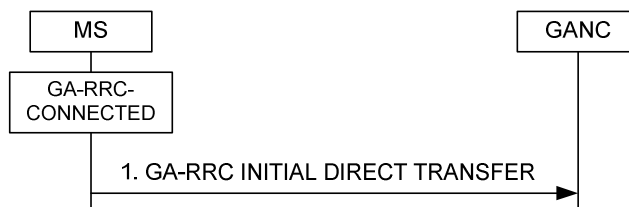
Figure 8a.2.1.1 Initial direct transfer, normal flow
