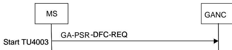
Figure 8.11.1: MS initiated Downlink Flow Control
