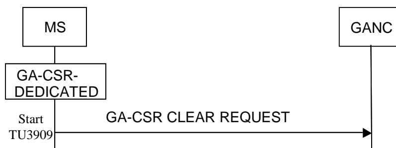
Figure 7.5.1.1 Initiation of GA-CSR connection release by MS
