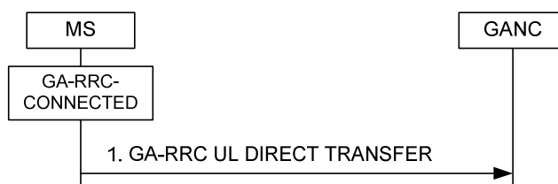
Figure 8a.2.3.1 Uplink direct transfer, normal flow
