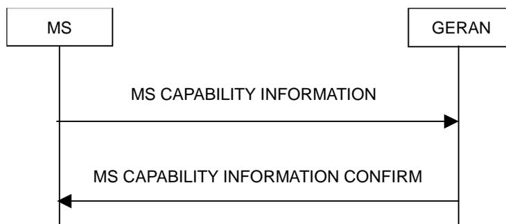
**Figure 7.6.1.1 : Transmission of MS capability information, normal flow**
