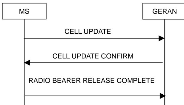
**Figure 7.8.1.3: Cell Update procedure with radio bearer release**
