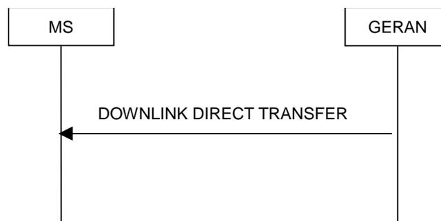
**Figure 7.17.2.1: Downlink Direct transfer, normal flow**
