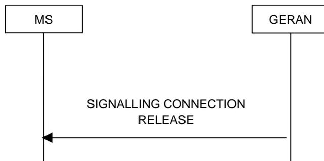
**Figure 7.15.1.1.1: Signalling Connection Release procedure, normal case**
