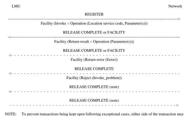
Figure 3.1: LMU initiated location service transaction
