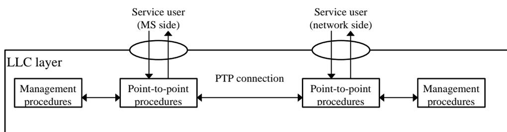
Figure C.1: Model of the LLC layer peer-to-peer procedures
