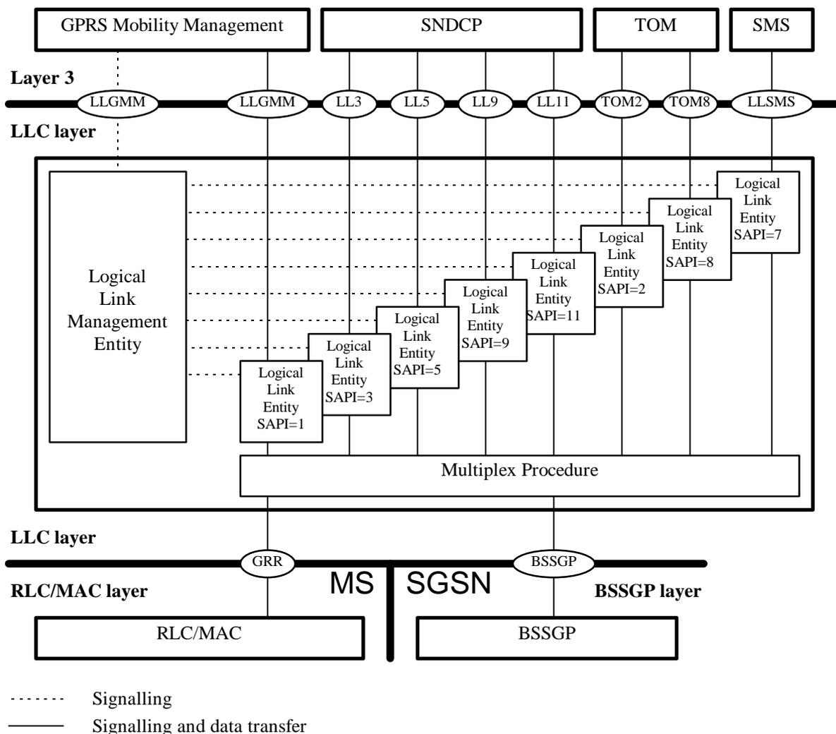
Figure 2: Functional model of the LLC layer
