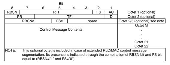
Figure 10.3.1.2: Downlink RLC/MAC control block message contents
