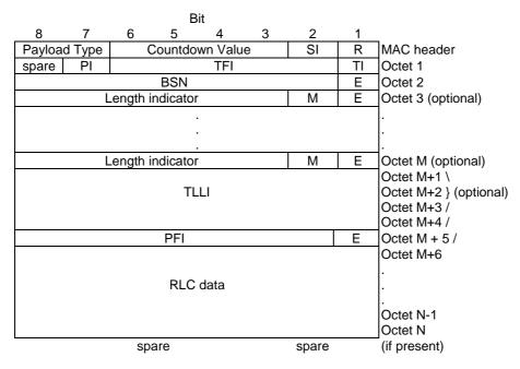
NOTE: The field mapping convention for GPRS (sub-clause 10.0b.3.1) applies. According to that, in particular regarding the TLLI field, the *most significant byte* of the TLLI value shall be mapped on octet M+1 and the *least significant byte* of the TLLI value shall be mapped on octet M+4 of the uplink RLC data block.
