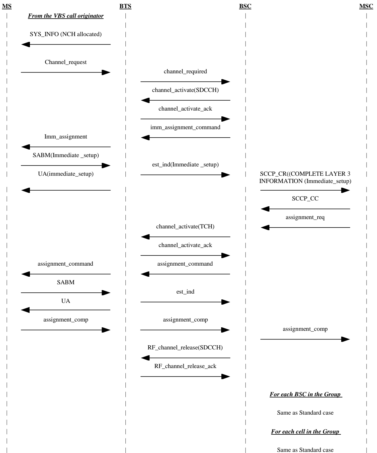
Figure 4a: Signalling information required for establishing voice broadcast calls by a service subscriber using immediate setup
