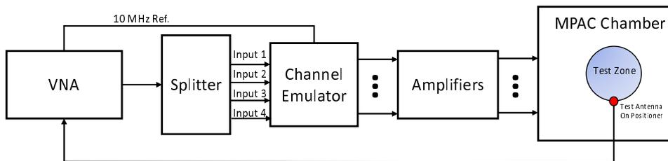
Figure C.3.4-3: Configuration for spatial correlation validation (CDL-C UMa)
