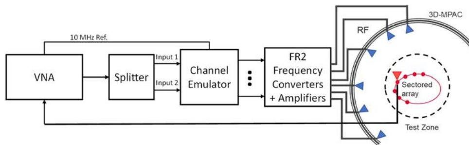
**Figure I.3.4-2: Setup for FR2 PSP validation measurements**
