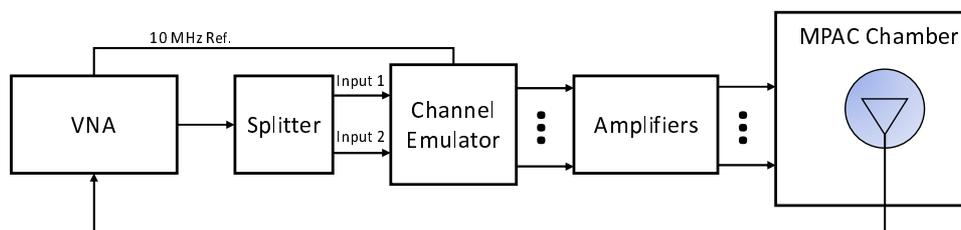
**Figure C.3.5-1: Setup for Beam-Specific V/H measurements (Beam 1)**
