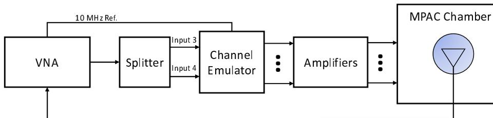
Figure C.3.5-2: Setup for Beam-Specific V/H measurements (Beam 2 CDL-C UMa only)
