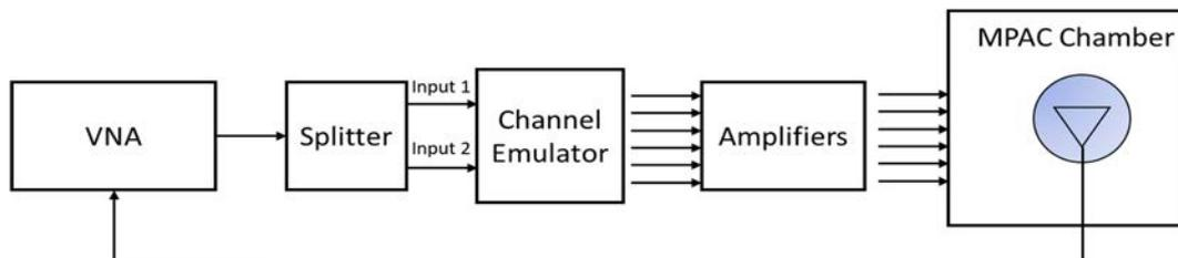
**Figure C.3.5-1: Setup for Beam-Specific V/H measurements (Beam 1)**
