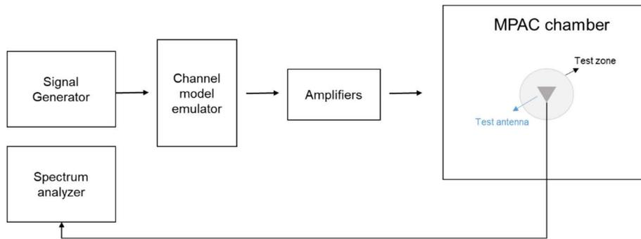
**Figure C.3.3-1: Setup for Doppler measurements**
