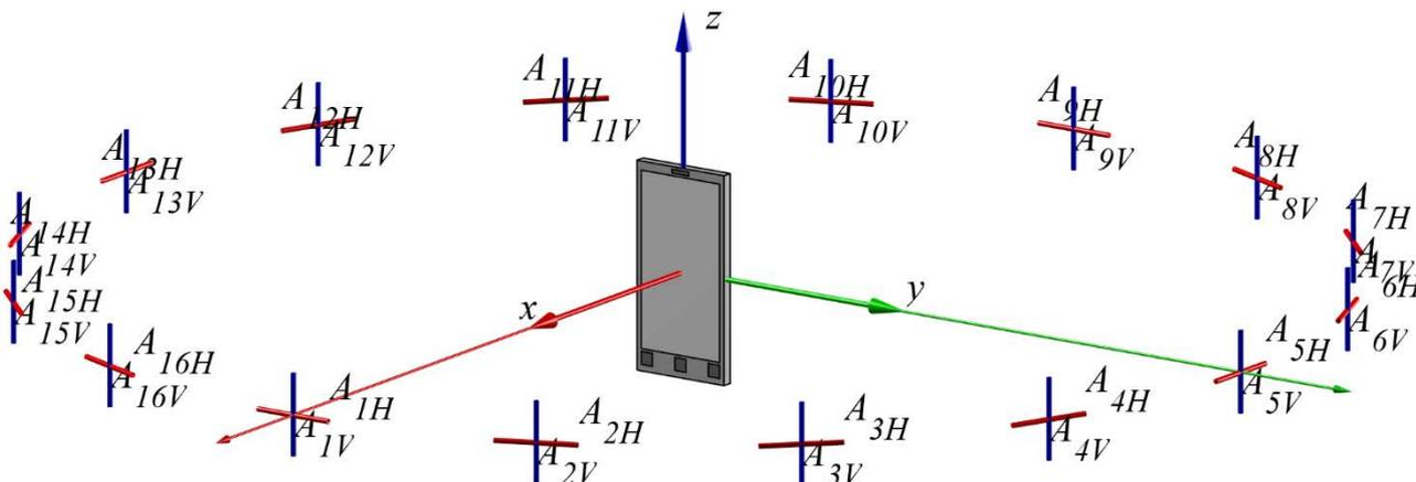
**Figure A.2.1-2: OTA chamber antenna setup with sixteen uniformly spaced dual polarized chamber antennas**
