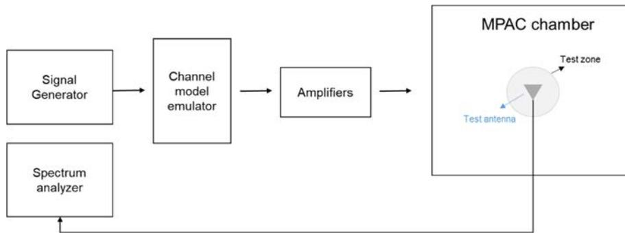
**Figure C.3.3-1: Setup for Doppler measurements**
