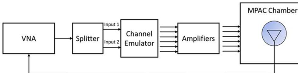
**Figure C.3.2-2: Setup for Beam-Specific PDP measurements (Beam 1)**
