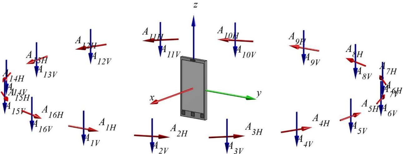
**Figure A.2.1-2: OTA chamber antenna setup with sixteen uniformly spaced dual polarized chamber antennas**
