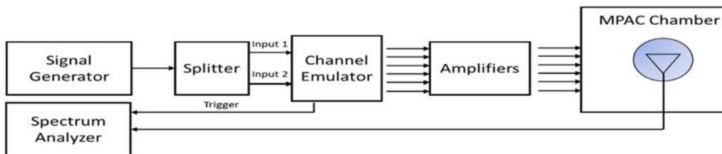
**Figure C.3.5-3: Setup for Beam-Specific V/H measurements (Beam 1)**
