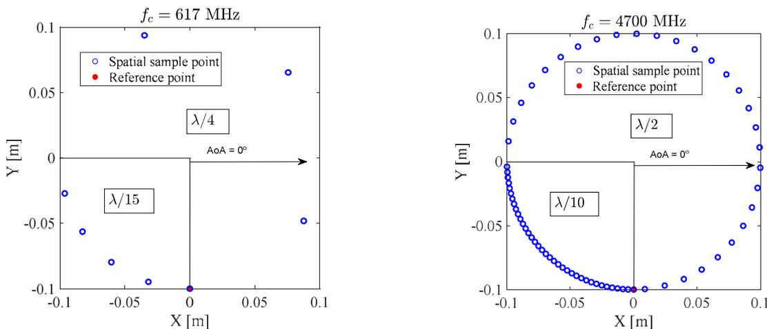
**Figure C.3.4-5: Spatial sampling for spatial correlation validation measurement for test frequencies less than and equal to or greater than 1800 MHz: 617 MHz spatial sampling (left) and 4700 MHz spatial sampling (right)**
