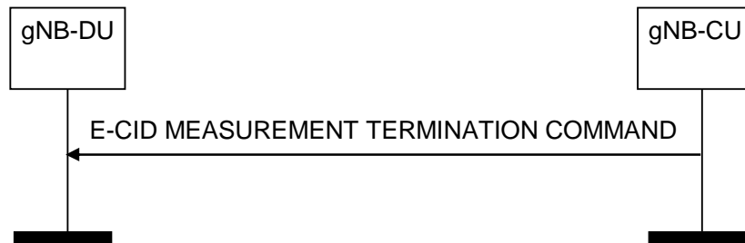
Figure 8.13.15.2-1: E-CID Measurement Termination procedure, successful operation
