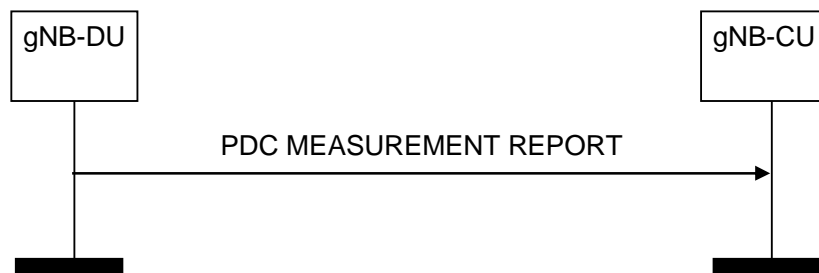
Figure 8.15.2.2-1: PDC Measurement Report procedure, successful operation
