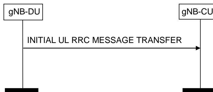
Figure 8.4.1.2-1: Initial UL RRC Message Transfer procedure.
