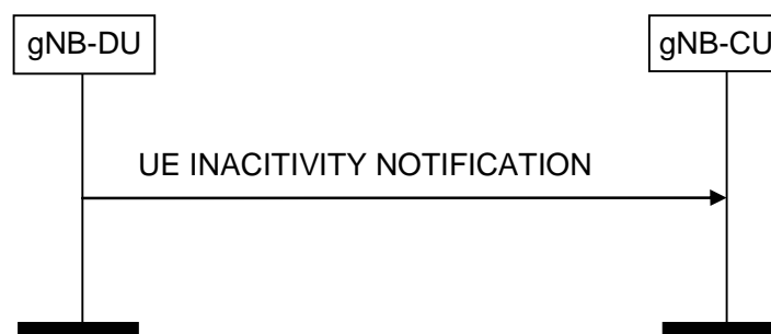
Figure 8.3.6.2-1: UE Inactivity Notification procedure.
