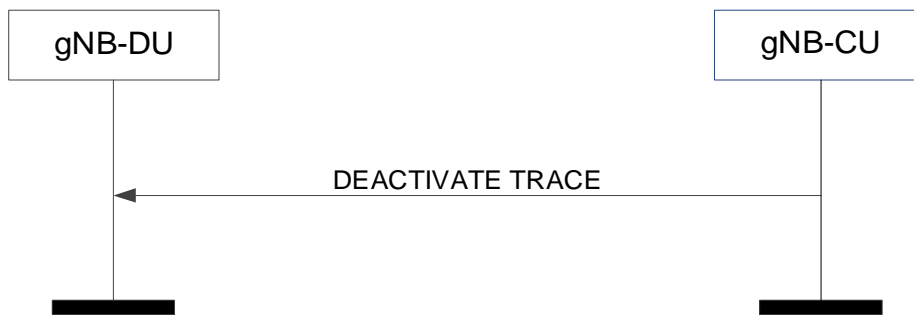
Figure 8.8.2.2-1: Deactivate trace procedure: Successful Operation
