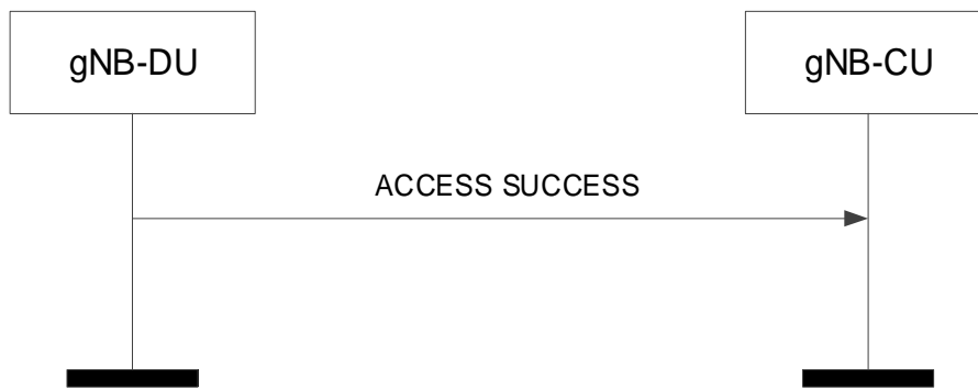
Figure 8.3.8.2-1: Access Success procedure. Successful operation.
