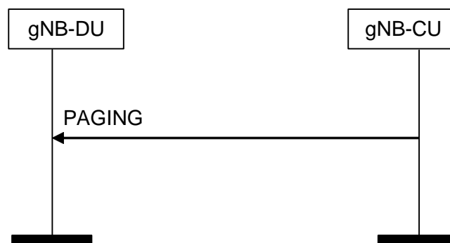
Figure 8.7.1.2-1: Paging procedure. Successful operation.
