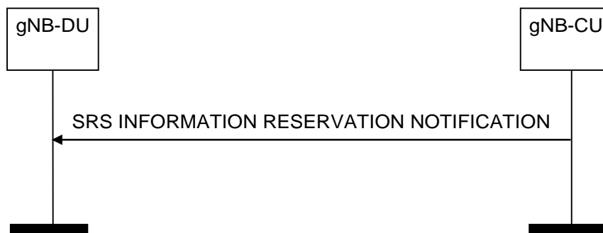
Figure 8.13.21.2-1: SRS Information Reservation Notification procedure, successful operation
