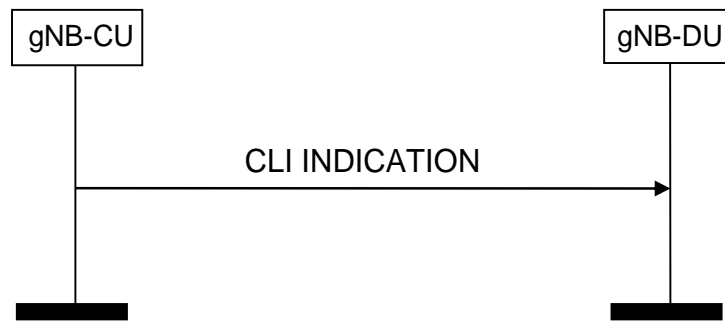
Figure 8.2.15.2-2: CLI Indication initiated from the gNB-CU, successful operation
