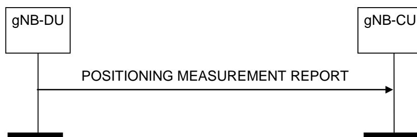
Figure 8.13.4.2-1: Positioning Measurement Report procedure: successful operation
