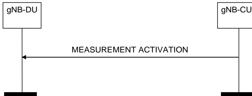
Figure 8.13.19.2-1: Measurement Activation procedure, successful operation
