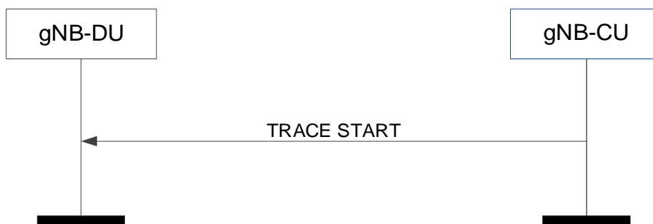
Figure 8.8.1.2-1: Trace start procedure: Successful Operation.
