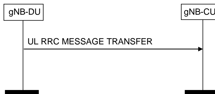
Figure 8.4.3.2-1: UL RRC Message Transfer procedure
