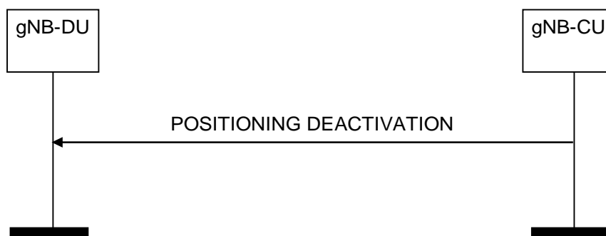
Figure 8.13.11.2-1: Positioning Deactivation procedure, successful operation
