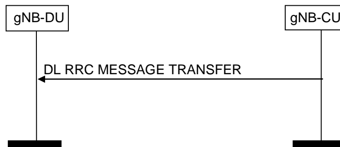
Figure 8.4.2.2-1: DL RRC Message Transfer procedure
