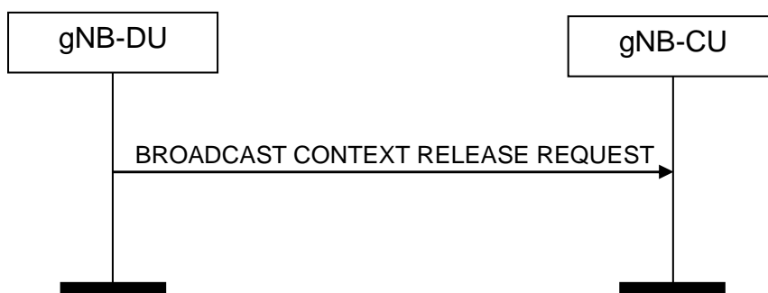
Figure 8.14.3.2-1: Broadcast Context Release Request procedure. Successful operation
