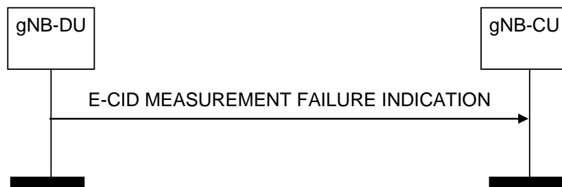
Figure 8.13.13.2-1: E-CID Measurement Failure Indication, successful operation
