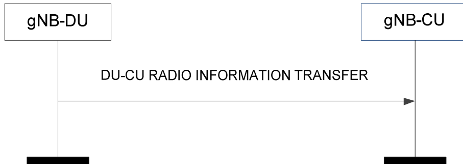
Figure 8.9.1.2-1: DU-CU Radio Information Transfer procedure.
