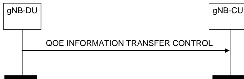
Figure 8.16.2.2-1: QoE Information Transfer Control procedure.
