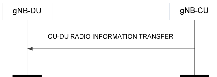
Figure 8.9.2.2-1: CU-DU Radio Information Transfer procedure.
