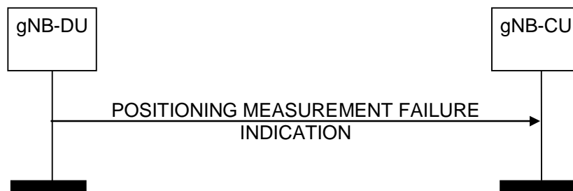
Figure 8.13.6.2-1: Positioning Measurement Failure Indication procedure: successful operation
