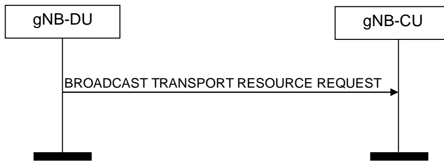
Figure 8.14.14.2-1: Broadcast Transport Resource Request procedure. Successful operation
