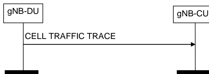
Figure 8.8.3.2-1: Cell Traffic Trace procedure. Successful operation.
