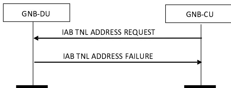
Figure 8.10.3.3-1: IAB TNL Address Allocation procedure: Unsuccessful Operation
