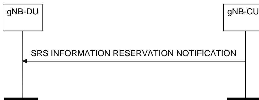
Figure 8.13.21.2-1: SRS Information Reservation Notification procedure, successful operation
