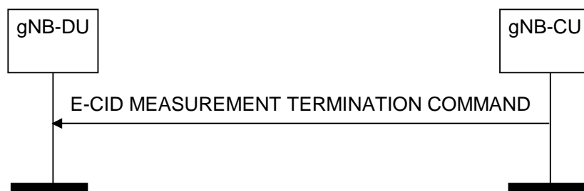
Figure 8.13.15.2-1: E-CID Measurement Termination procedure, successful operation
