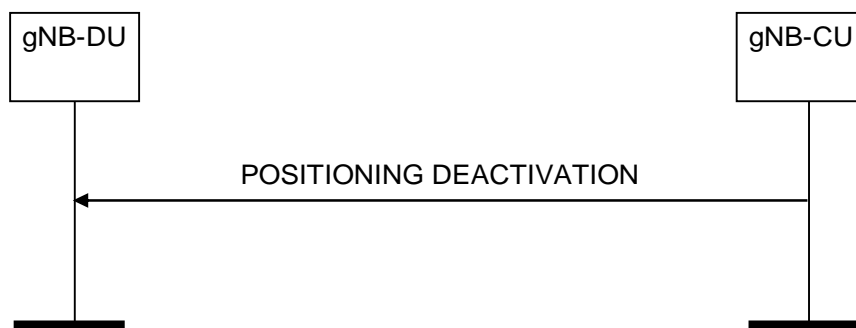
Figure 8.13.11.2-1: Positioning Deactivation procedure, successful operation
