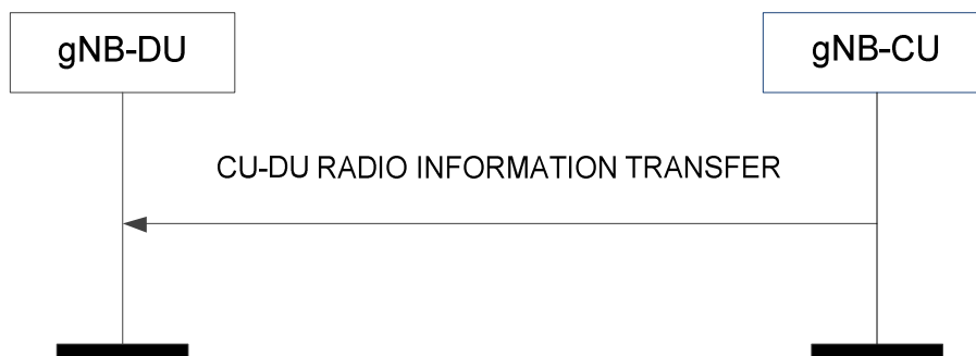
Figure 8.9.2.2-1: CU-DU Radio Information Transfer procedure.
