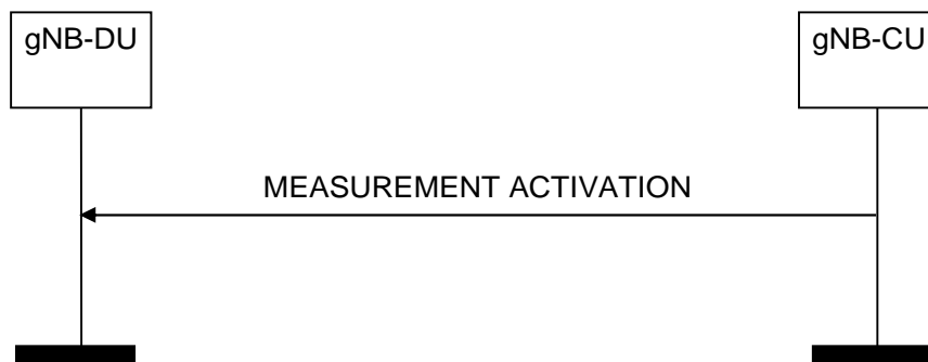
Figure 8.13.19.2-1: Measurement Activation procedure, successful operation
