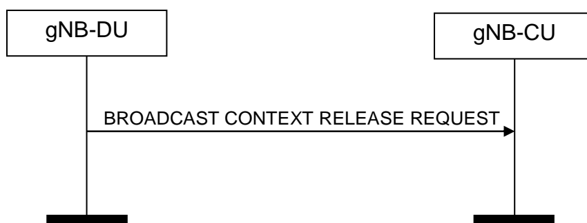
Figure 8.14.3.2-1: Broadcast Context Release Request procedure. Successful operation
