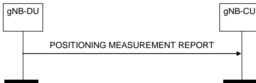
Figure 8.13.4.2-1: Positioning Measurement Report procedure: successful operation
