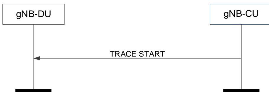
Figure 8.8.1.2-1: Trace start procedure: Successful Operation.
