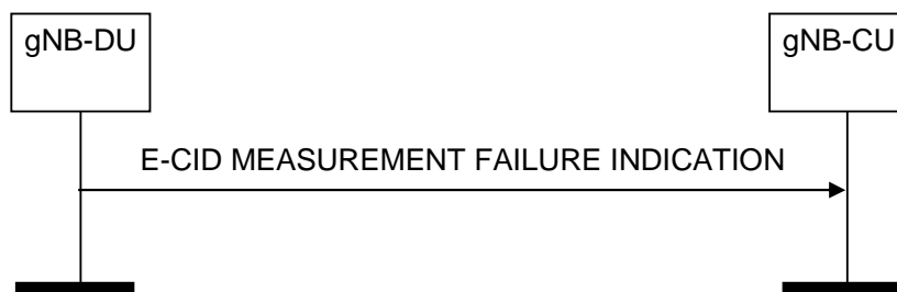
Figure 8.13.13.2-1: E-CID Measurement Failure Indication, successful operation
