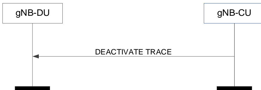
Figure 8.8.2.2-1: Deactivate trace procedure: Successful Operation
