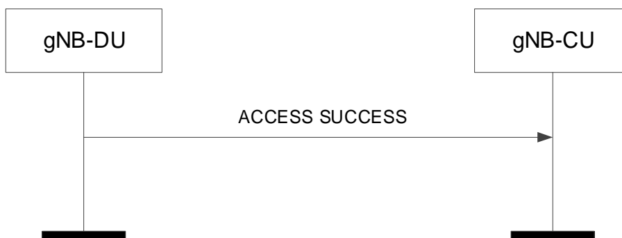
Figure 8.3.8.2-1: Access Success procedure. Successful operation.
