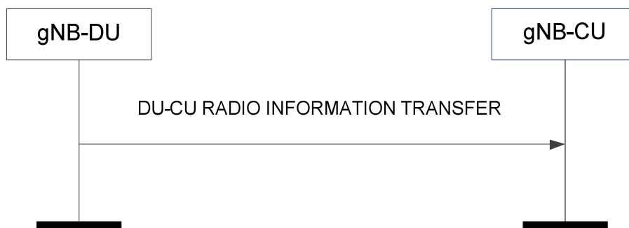
Figure 8.9.1.2-1: DU-CU Radio Information Transfer procedure.
