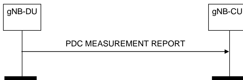
Figure 8.15.2.2-1: PDC Measurement Report procedure, successful operation
