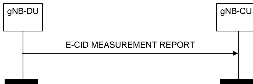
Figure 8.13.14.2-1: E-CID Measurement Report procedure, successful operation
