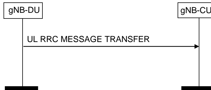
Figure 8.4.3.2-1: UL RRC Message Transfer procedure
