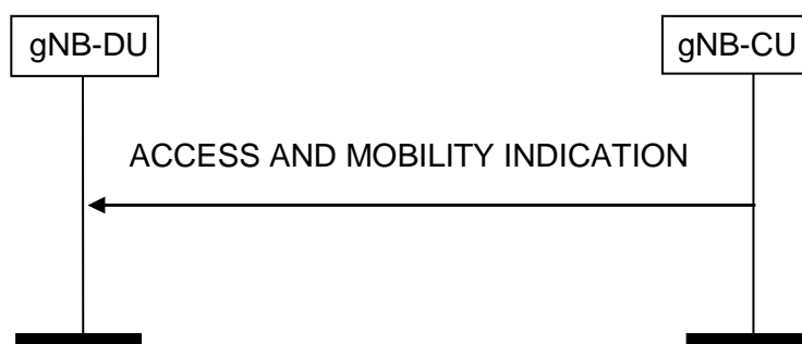
Figure 8.11.1.2-1: Access and Mobility Indication procedure. Successful operation
