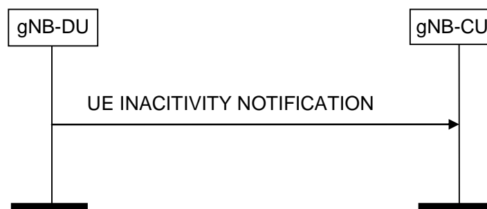
Figure 8.3.6.2-1: UE Inactivity Notification procedure.
