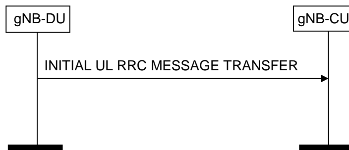
Figure 8.4.1.2-1: Initial UL RRC Message Transfer procedure.
