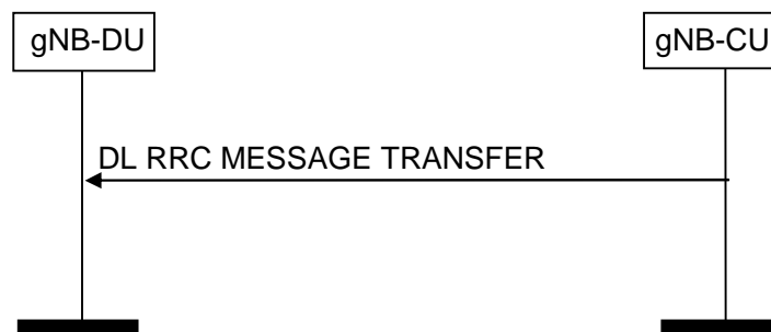
Figure 8.4.2.2-1: DL RRC Message Transfer procedure
