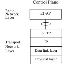
Figure 7.1-1: Interface protocol structure for E1
