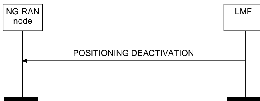
Figure 8.2.10.2-1: Positioning Deactivation procedure, successful operation
