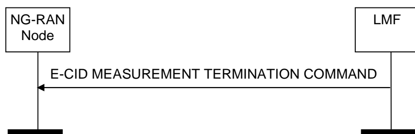
Figure 8.2.4.2-1: E-CID Measurement Termination procedure, successful operation
