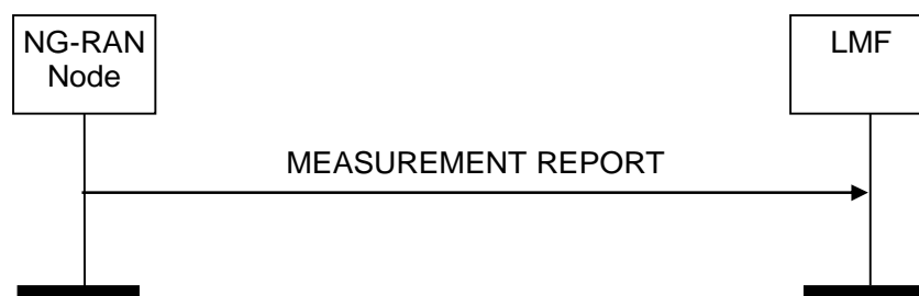
Figure 8.5.2.2.1: Measurement Report procedure. Successful operation.
