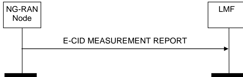
Figure 8.2.3.2-1: E-CID Measurement Report procedure, successful operation
