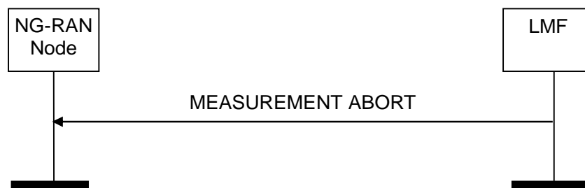
Figure 8.5.4.2.1: Measurement Abort Procedure: Successful Operation.
