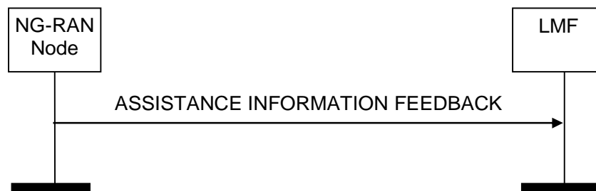
Figure 8.4.2.2-1: Assistance Information Feedback procedure
