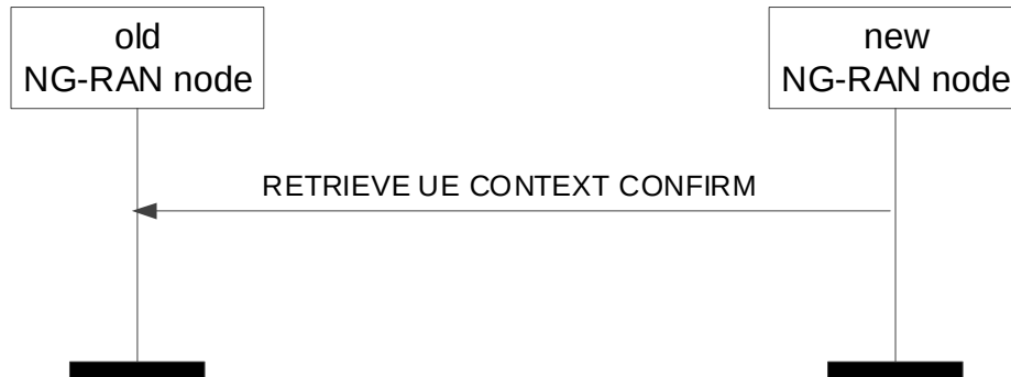
Figure 8.2.12.2-1: Retrieve UE Context Confirm, successful operation
