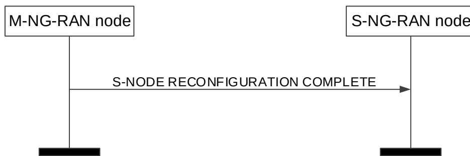
Figure 8.3.2.2-1: S-NG-RAN node Reconfiguration Complete procedure, successful operation.
