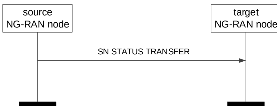
Figure 8.2.2.2-1: SN Status Transfer, successful operation
