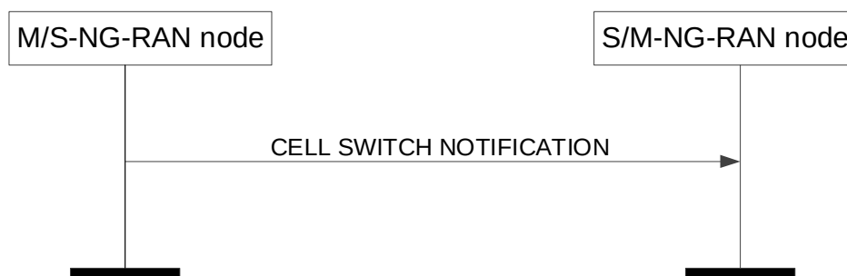
Figure 8.6.3.2-2: Cell Switch Notification procedure for dual connectivity. Successful operation.
