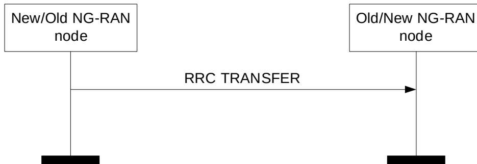
Figure 8.3.9.2-2: RRC Transfer procedure for SDT, successful operation.
