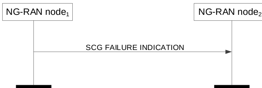
Figure 8.4.16.2-1: SCG Failure Indication, successful operation
