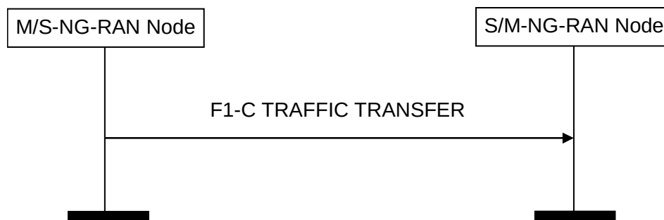
Figure 8.5.1.2-1: F1-C Traffic Transfer procedure, successful operation
