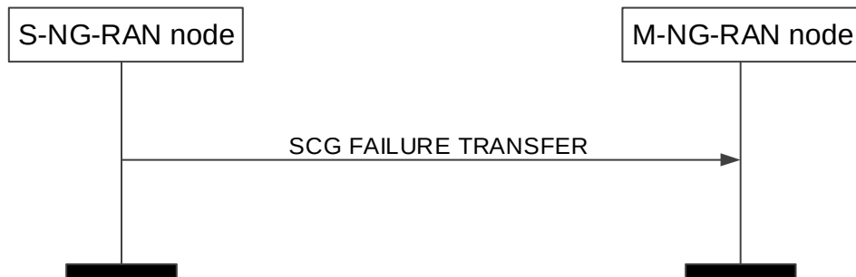
Figure 8.3.18.2-1: SCG Failure Information Transfer, successful operation
