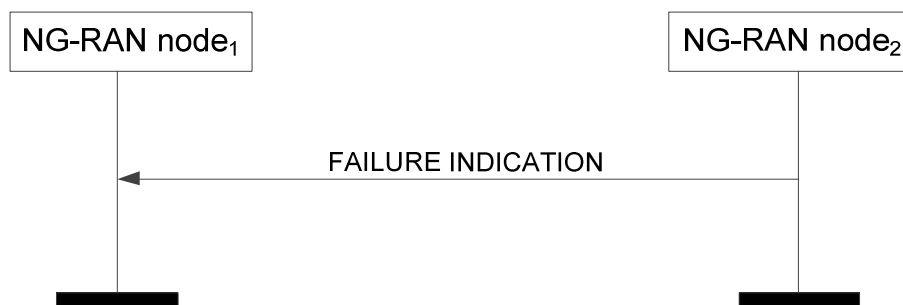
Figure 8.4.7.2-1: Failure Indication, successful operation
