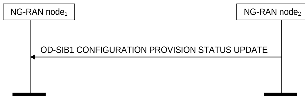
Figure 8.4.18.2-1: OD-SIB1 Configuration Provision Status Update procedure, successful operation
