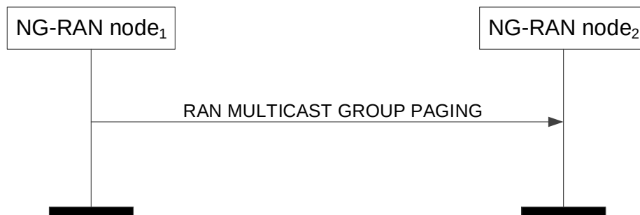
Figure 8.2.11.2-1: RAN Multicast Group Paging, successful operation
