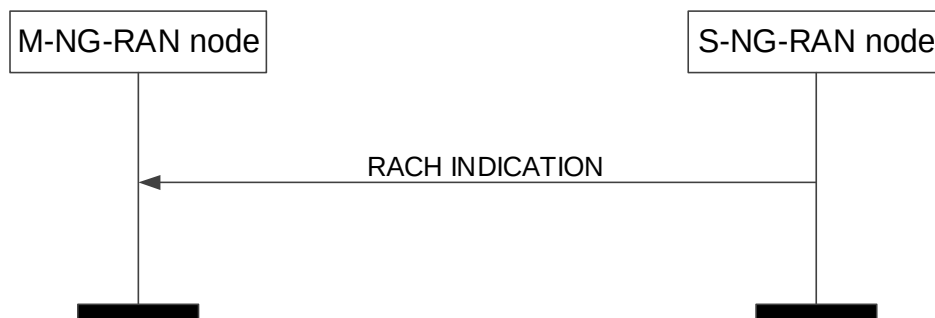
Figure 8.3.20.2-1: RACH Indication procedure, successful operation.
