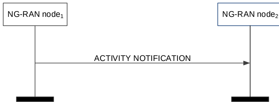
Figure 8.3.11.2-1: Activity Notification, successful operation
