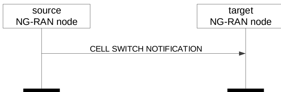
Figure 8.6.3.2-1: Cell Switch Notification procedure. Successful operation.
