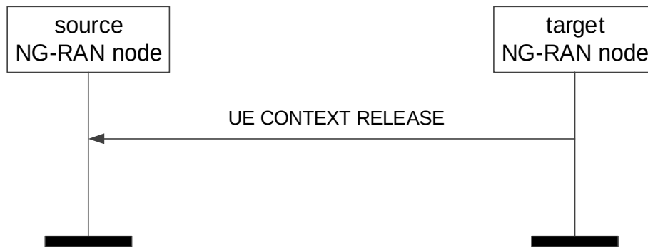
Figure 8.2.7.2-1: UE Context Release, successful operation for handover
