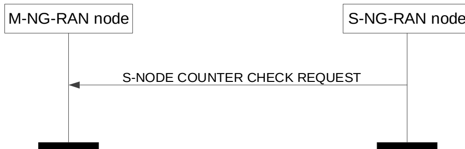
Figure 8.3.8.2-1: S-NG-RAN node Counter Check procedure, successful operation.
