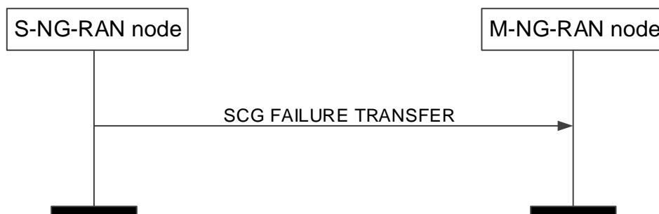
Figure 8.3.18.2-1: SCG Failure Information Transfer, successful operation
