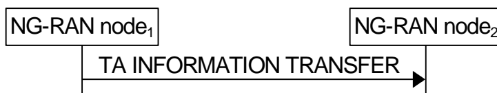
Figure 8.6.2.2-1: TA Information Transfer procedure. Successful operation.
