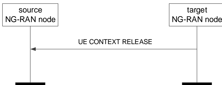
Figure 8.2.7.2-1: UE Context Release, successful operation for handover
