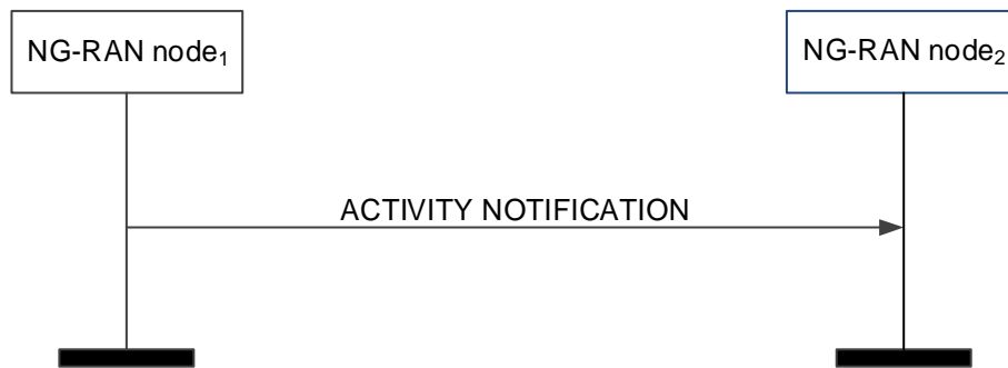
Figure 8.3.11.2-1: Activity Notification, successful operation
