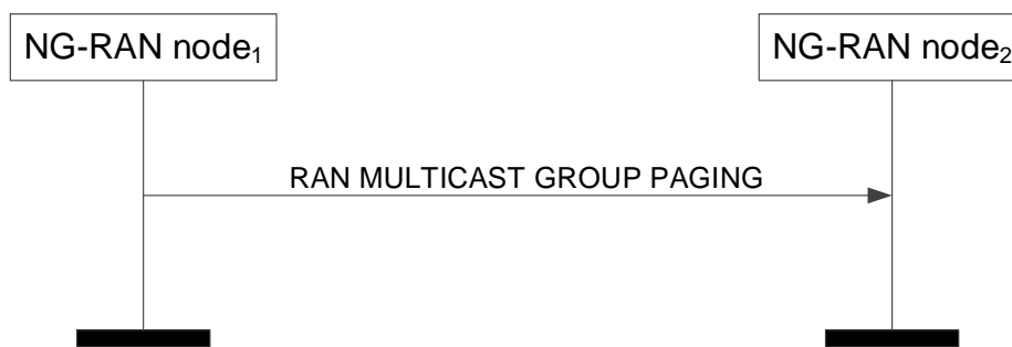
Figure 8.2.11.2-1: RAN Multicast Group Paging, successful operation
