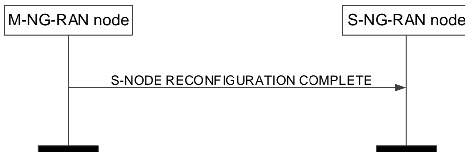
Figure 8.3.2.2-1: S-NG-RAN node Reconfiguration Complete procedure, successful operation.
