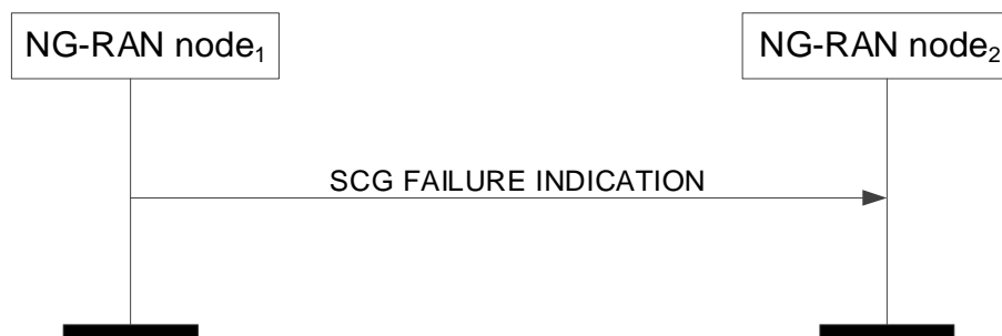
Figure 8.4.16.2-1: SCG Failure Indication, successful operation
