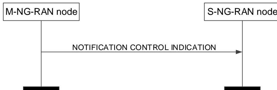
Figure 8.3.10.2-1: Notification Control Indication procedure, M-NG-RAN node initiated, successful operation.
