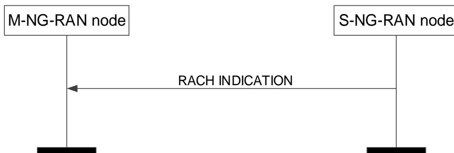
Figure 8.3.20.2-1: RACH Indication procedure, successful operation.
