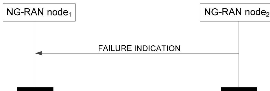
Figure 8.4.7.2-1: Failure Indication, successful operation
