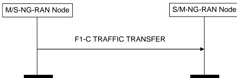
Figure 8.5.1.2-1: F1-C Traffic Transfer procedure, successful operation
