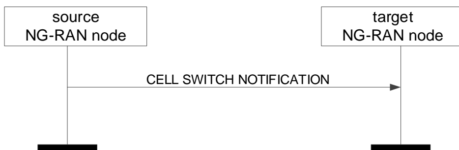
Figure 8.6.3.2-1: Cell Switch Notification procedure. Successful operation.
