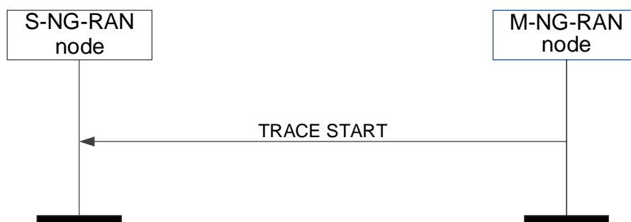
Figure 8.3.14.2-1: Trace Start, successful operation
