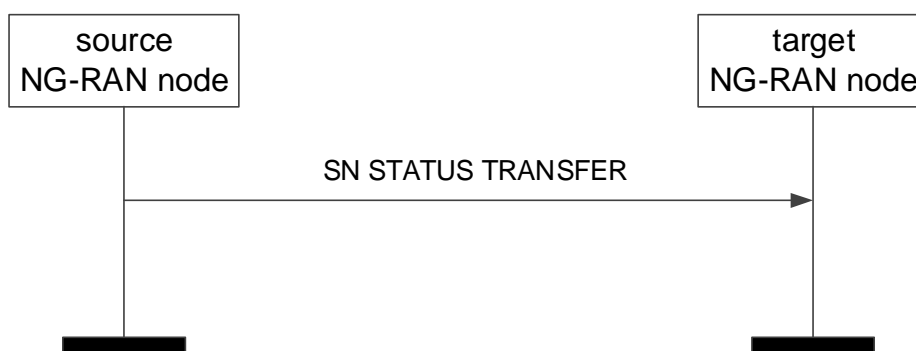
Figure 8.2.2.2-1: SN Status Transfer, successful operation
