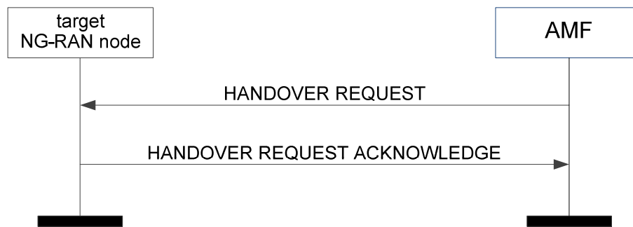
Figure 8.4.2.2-1: Handover resource allocation: successful operation
