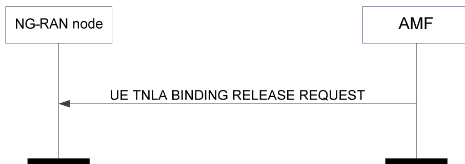
Figure 8.13.1.2-1: UE TNLA binding release request
