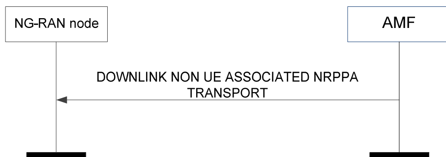
Figure 8.10.2.3-1: Downlink non UE-associated NRPPa transport
