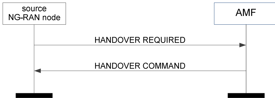
Figure 8.4.1.2-1: Handover preparation: successful operation
