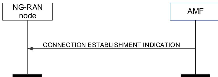
**Figure 8.3.6.2-1: Connection Establishment Indication procedure. Successful operation.**
