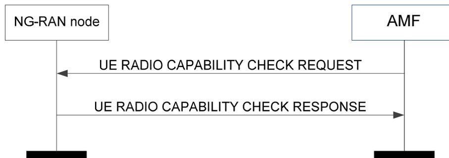
**Figure 8.14.2.2-1: UE radio capability check procedure: successful operation**
