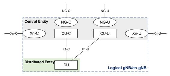
Figure A-1: Example deployment of an Logical gNB/en-gNB
