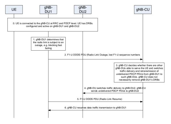
Figure 8.3.1-1: Procedure for centralized retransmission in intra gNB-CU scenarios
