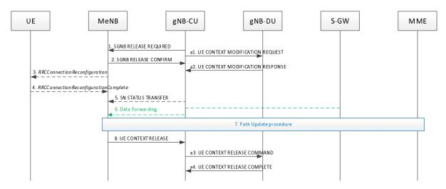
Figure 8.4.2.1-2 SgNB release procedure in EN-DC (SN initiated)
