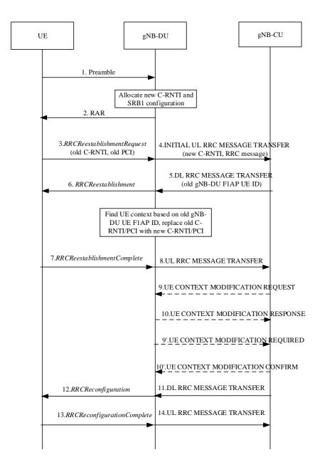
Figure 8.7-1: RRC connection reestablishment procedure
