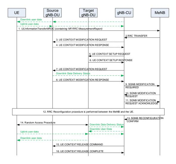
Figure 8.2.2.1-1: Inter-gNB-DU Mobility using MCG SRB in EN-DC
