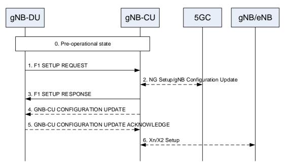
Figure 8.5-1: F1 startup and cell activation
