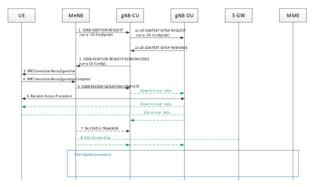
Figure 8.4.1.1-1: SgNB addition procedure in EN-DC
