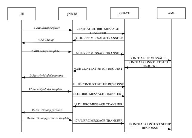
Figure 8.1-1: UE Initial Access procedure
