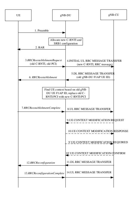
Figure 8.7-1: RRC connection reestablishment procedure
