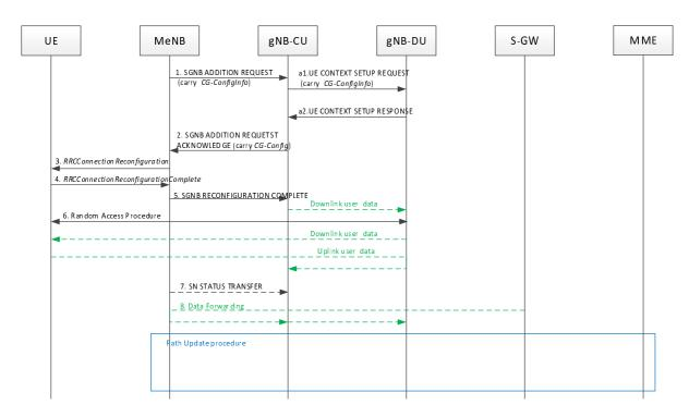
Figure 8.4.1.1-1: SgNB addition procedure in EN-DC
