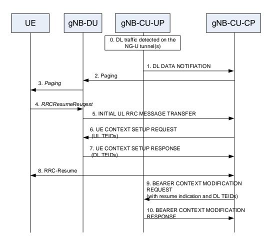
Figure 8.9.6.2-1: RRC Inactive to RRC Connected state transition.
