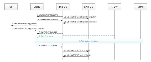
Figure 8.4.2.1-2 SgNB release procedure in EN-DC (SN initiated)
