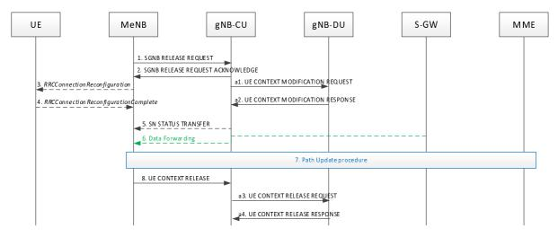
Figure 8.4.2.1-1 SgNB release procedure in EN-DC (MN initiated)
