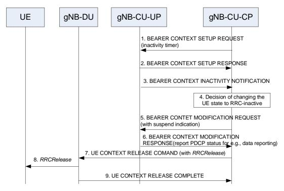
Figure 8.9.6.1-1: RRC Connected to RRC Inactive state transition.
