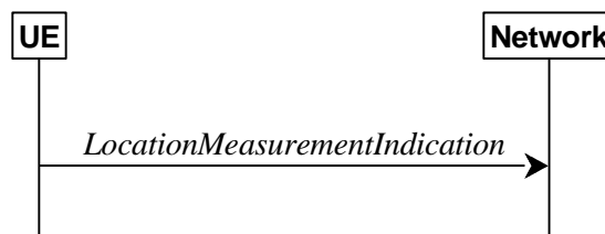
Figure 5.5.6.1-1: Location measurement indication
