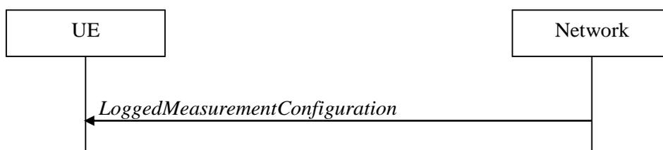
**Figure 5.5a.1.1-1: Logged measurement configuration**
