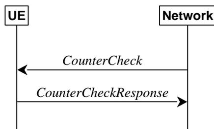
**Figure 5.3.6.1-1: Counter check procedure**
