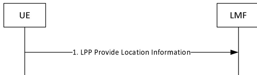
**Figure 8.2.3.3.2-1: UE-initiated Location Information Delivery Procedure.**
