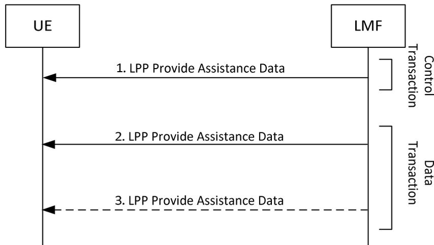
**Figure 8.1.3.2.1a-1: LPP Periodic Assistance data delivery procedure**
