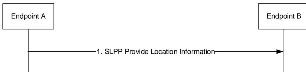
**Figure 7.11.2.3-2: SLPP Location Information Delivery procedure**
