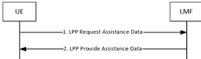
**Figure 8.12.3.1.2.2-1: UE-initiated Assistance Data Transfer Procedure**
