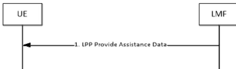
**Figure 8.6.3.2.1-1: LMF-initiated Assistance Data Delivery Procedure**
