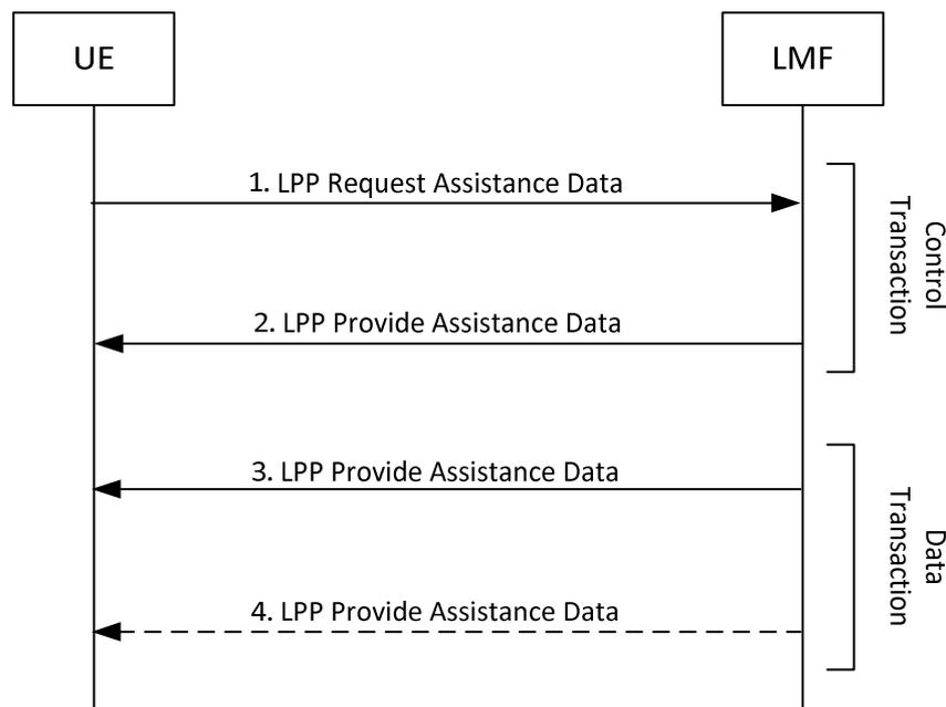
**Figure 8.12.3.1.2.2a-1: UE-initiated Periodic Assistance Data Transfer Procedure**
