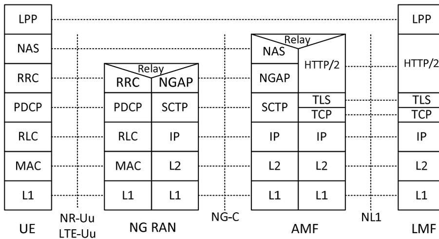
Figure 6.4.1-1: Protocol Layering for LMF to UE Signalling
