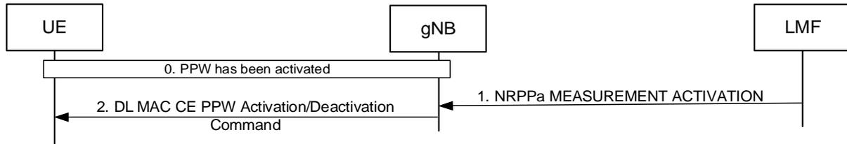
**Figure 7.8.2-2: Pre-configured PRS processing window deactivation procedure**
