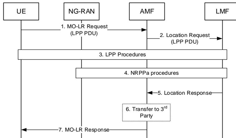
**Figure 7.3.3-1: UE Positioning Operations to support an MO-LR**
