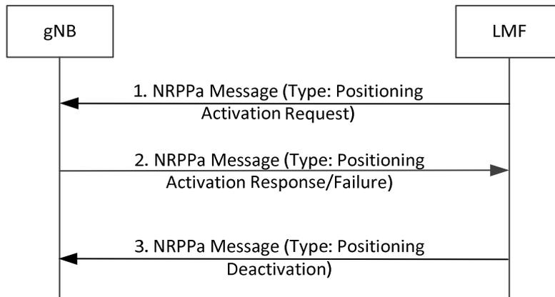
**Figure 8.14.3.3a-1: Positioning Activation/Deactivation Procedure.**
