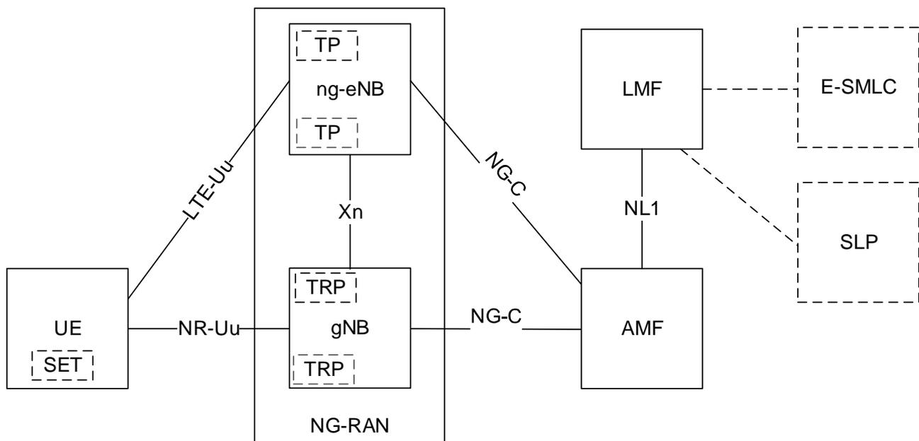
**Figure 5.1-1: UE Positioning Overall Architecture applicable to NG-RAN**
